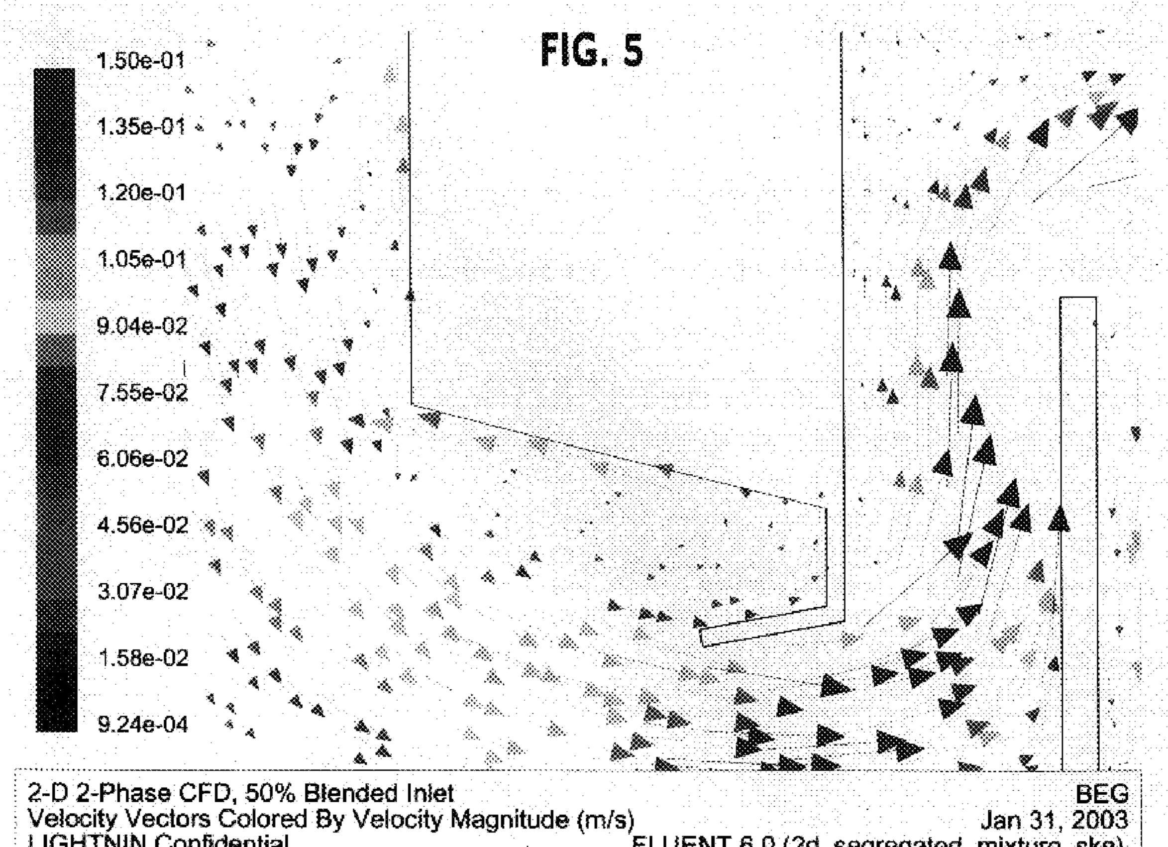
2-D 2-Phase CFD, 50% Blended Inlet Velocity Vectors Colored By Velocity Magnitude (m/s) LIGHTNIN Confidential 's)
