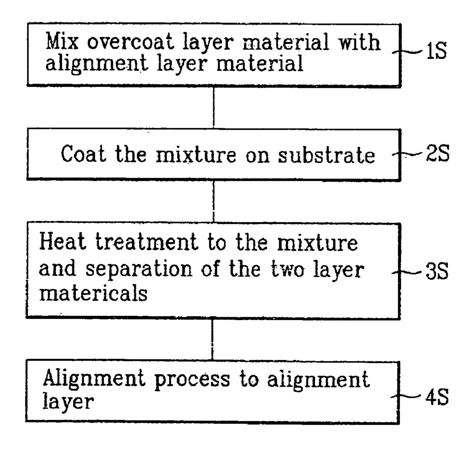
METHOD OF FORMING AN ALIGNMENT LAYER AND AN OVERCOAT LAYER IN A STACK STRUCTURE ON A SUBSTRATE OF A LIQUID CRYSTAL DISPLAY BY SEPARATING A MIXTURE OF AN ALIGNMENT LAYER MATERIAL FROM AN OVERCOAT LAYER MATERIAL IN A THERMAL CURING TREATMENT
