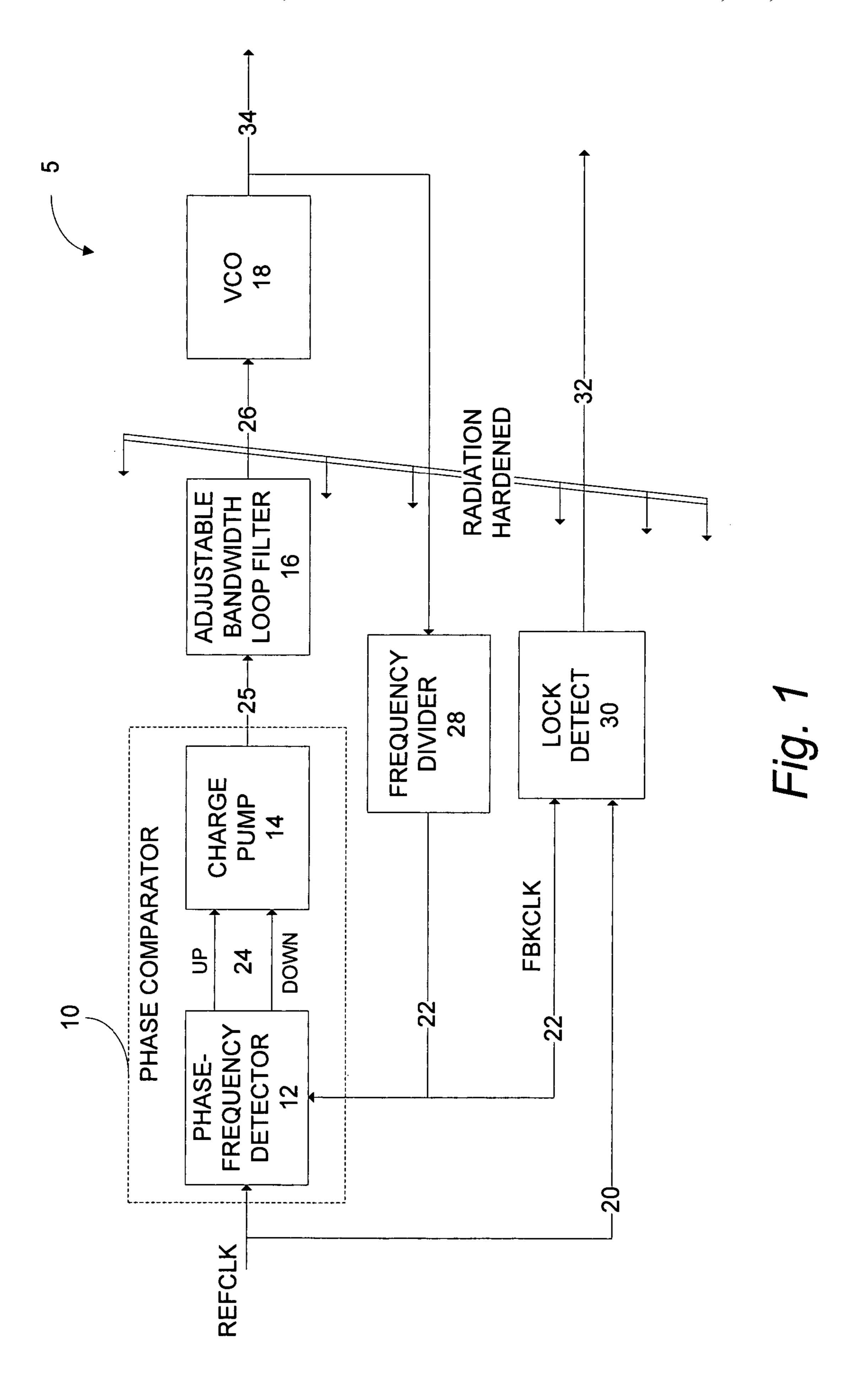
If a radiation event occurs, adjust the bandwidth of the adjustable filter to a narrow bandwidth
