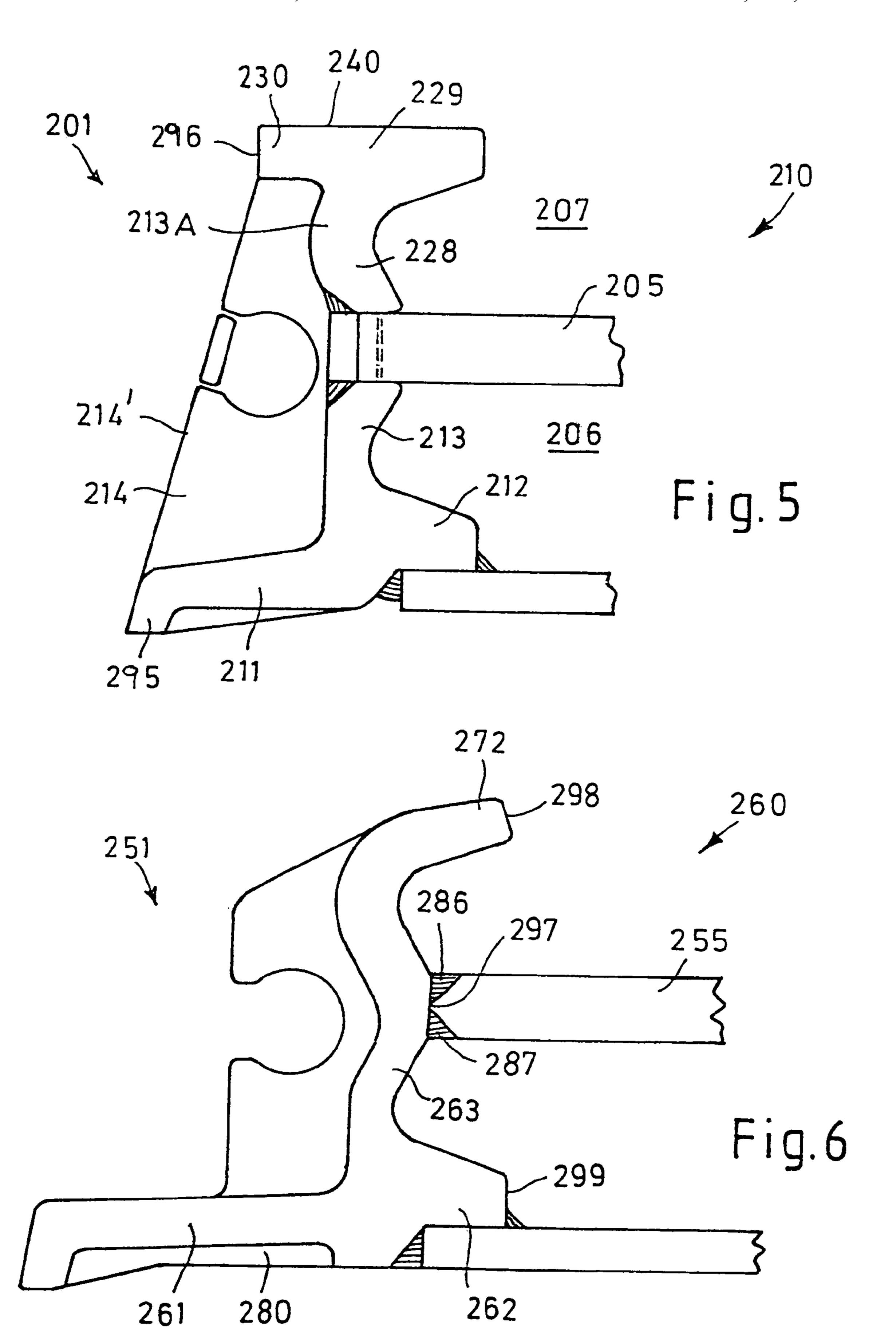
The present invention relates to a conveyor pan for underground face or gate conveyors, with a pair of side parts comprising cast parts which include cast vertical arms 5 extending over the height of the bottom run and the top run, a lower cast flange arm extending outwards to the rear, a cast foot flange extending inwards onto whose lower side a base plate is welded which closes the bottom run to the bottom, as well as on the end faces cast accepting elements for the 10
