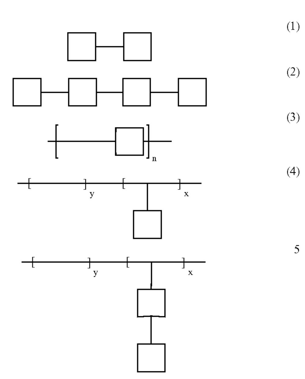
in which the continuous line is the main chain of the siloxane polymer and the squares represent the groups capable of establishing hydrogen interactions.
