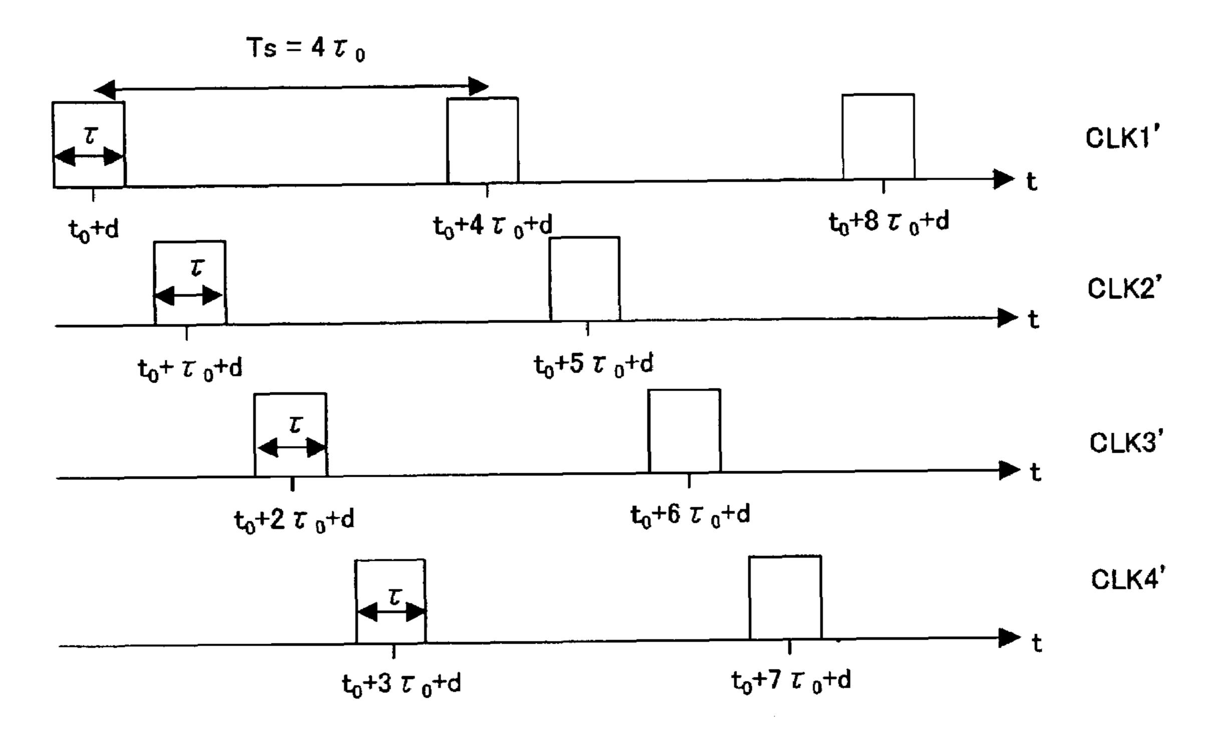
Sampling rate, fs = 1/Ts > 2 \* signal bandwidth
