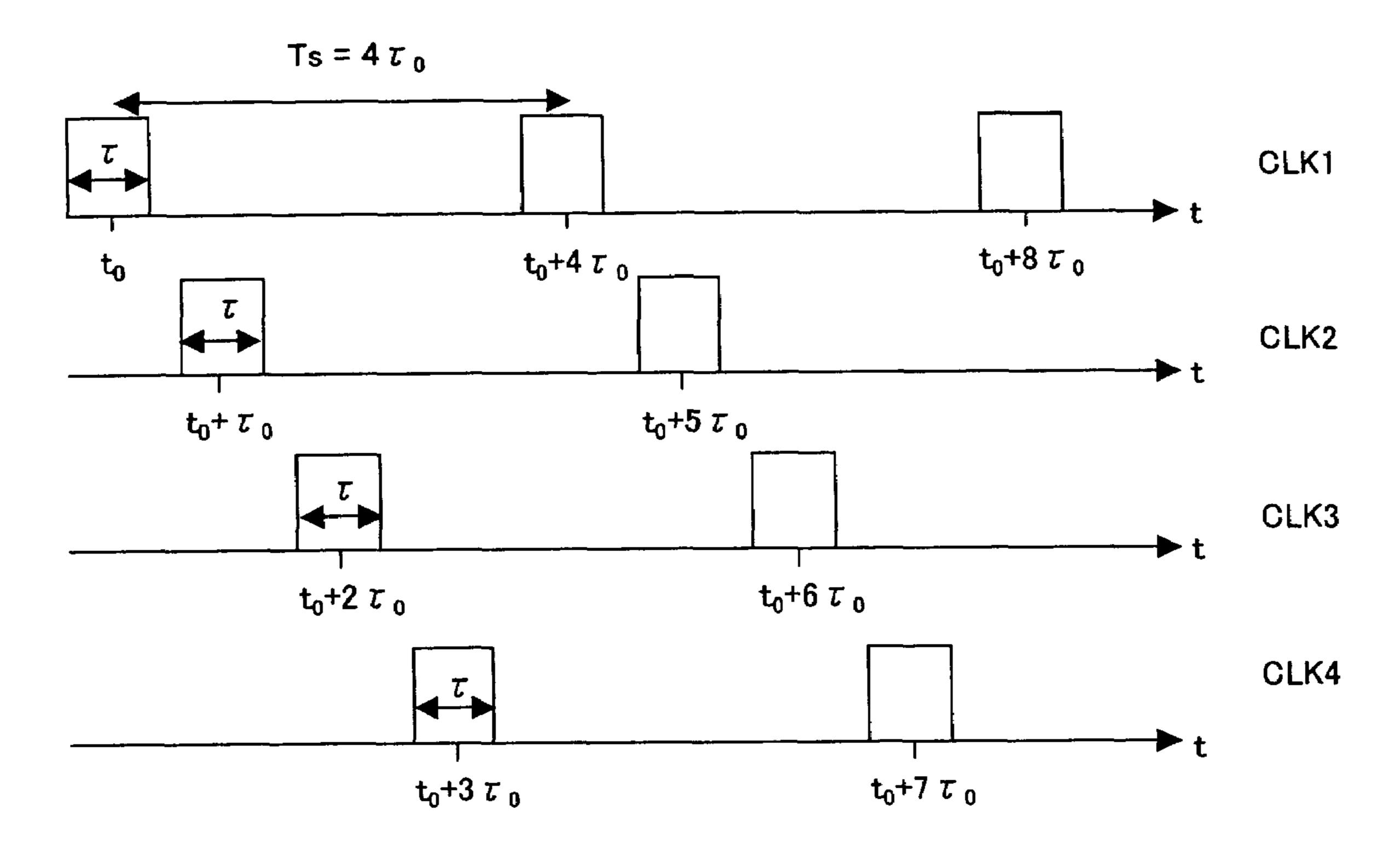
Sampling rate, fs = 1/Ts > 2 \* signal bandwidthPulse width,  $\tau \le \tau_0 = Ts / 4$
