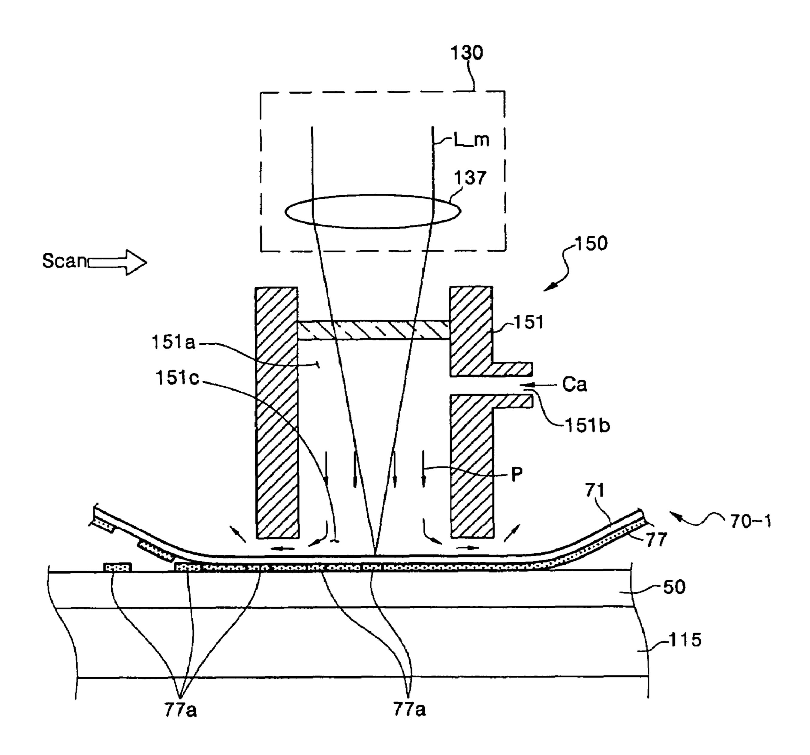
LASER INDUCED THERMAL IMAGING APPARATUS, LASER INDUCED THERMAL IMAGING METHOD USING THE APPARATUS, AND METHOD OF FABRICATING ORGANIC LIGHT EMITTING DISPLAY USING THE APPARATUS
