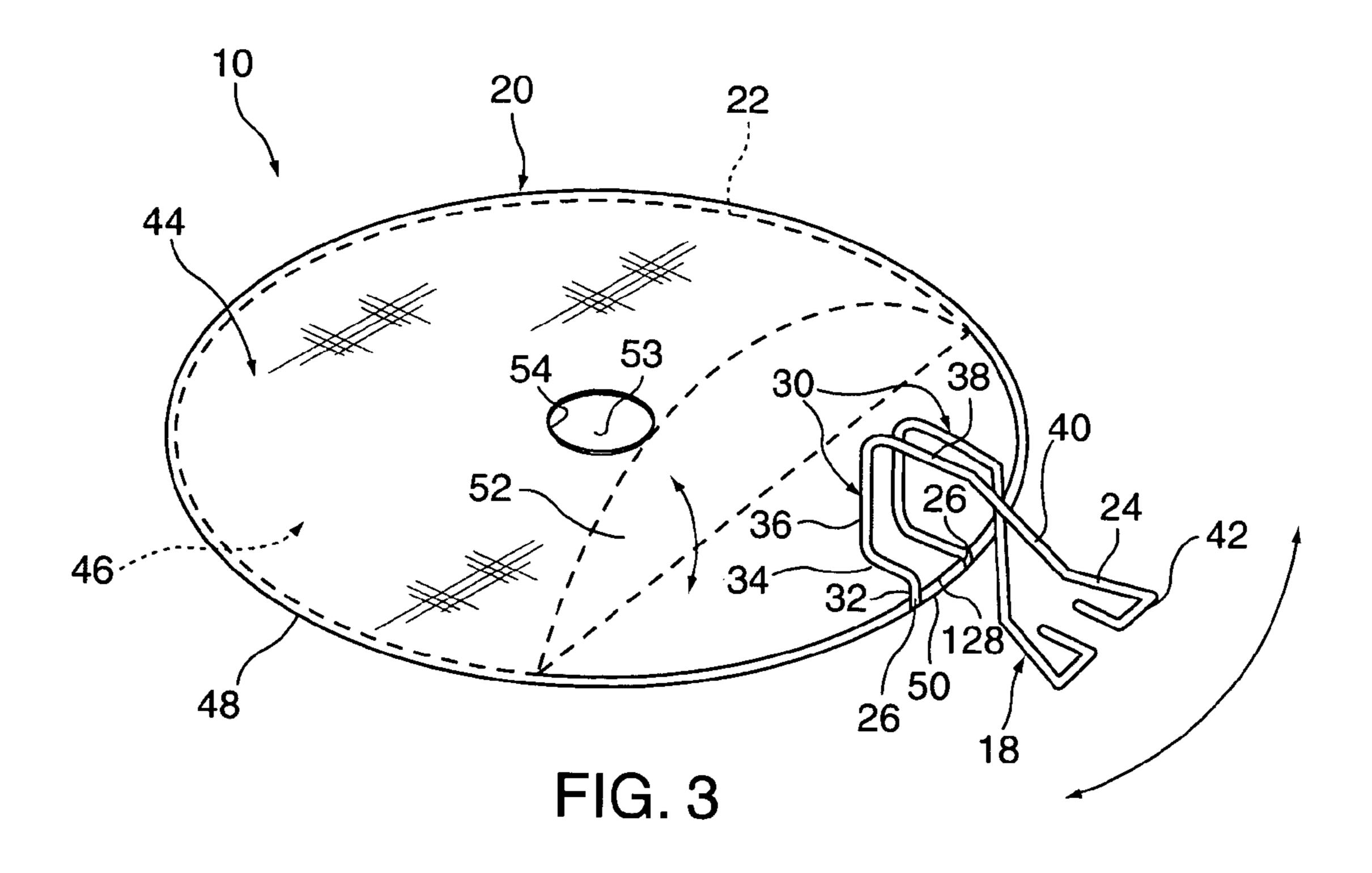
DISPOSABLE PROTECTOR FOR ENGAGING A CLOGGED TOILET AND CONTAINING SPLASHES IN THE CLOGGED TOILET OCCURRING DURING UNCLOGGING OF THE CLOGGED TOILET BY A PLUNGER
