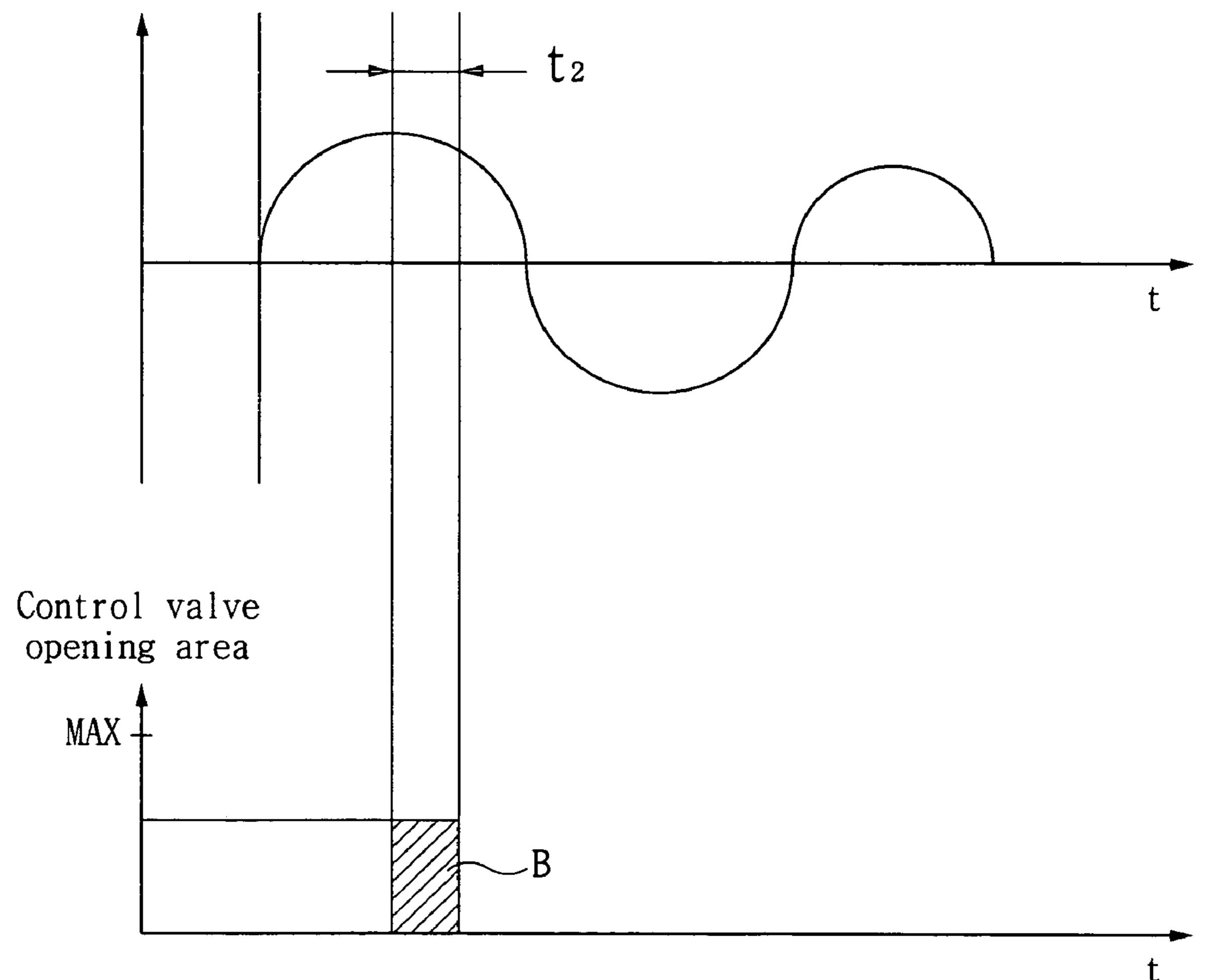
B: Supply fluid to small chamber and return fluid of large chamber to tank
