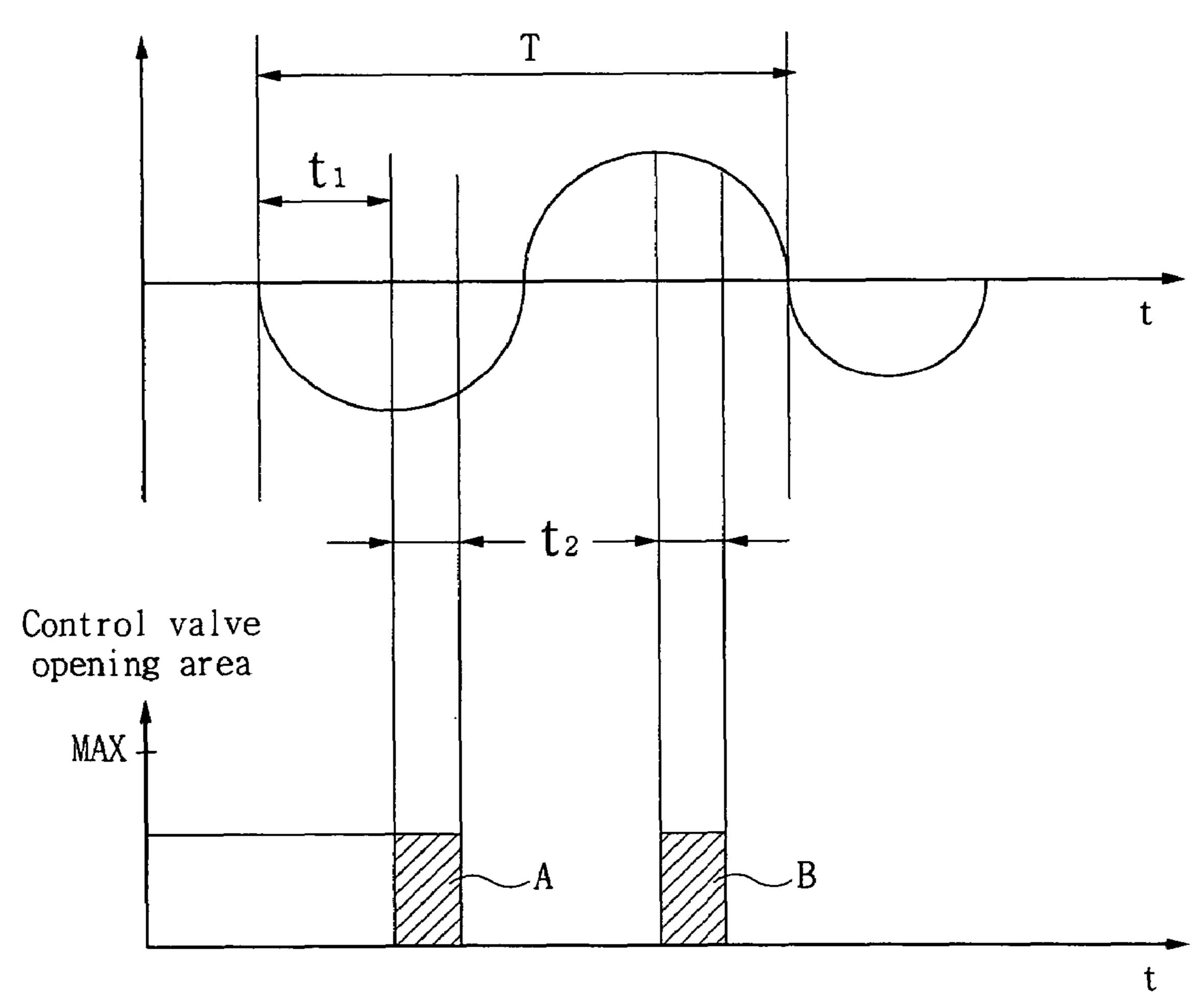
A: Supply fluid to large chamber and return fluid of small chamber to tank
