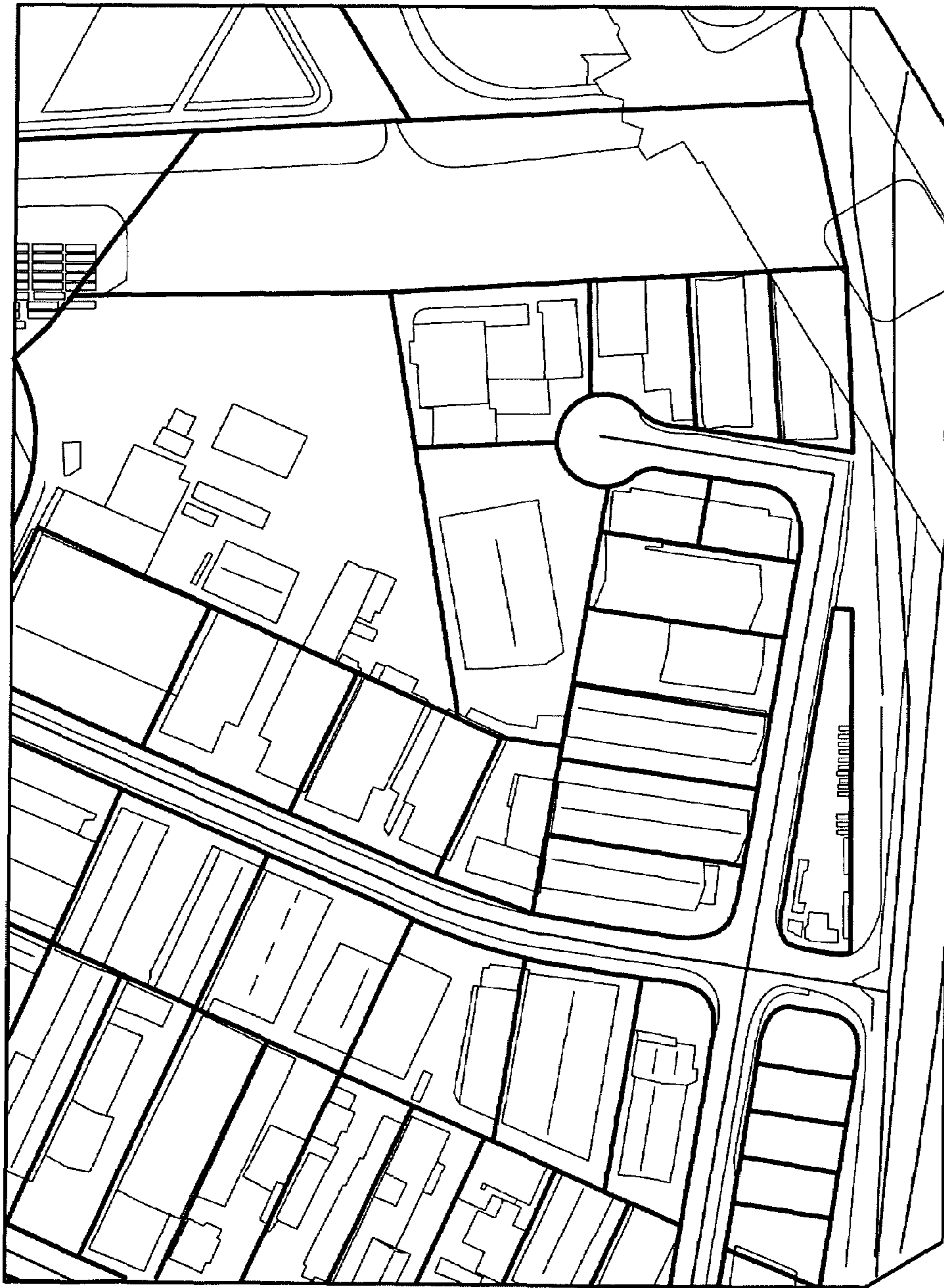
Sample of a Scaled and Georeferenced Aerial Photograph Overlaid onto a GIS Map
