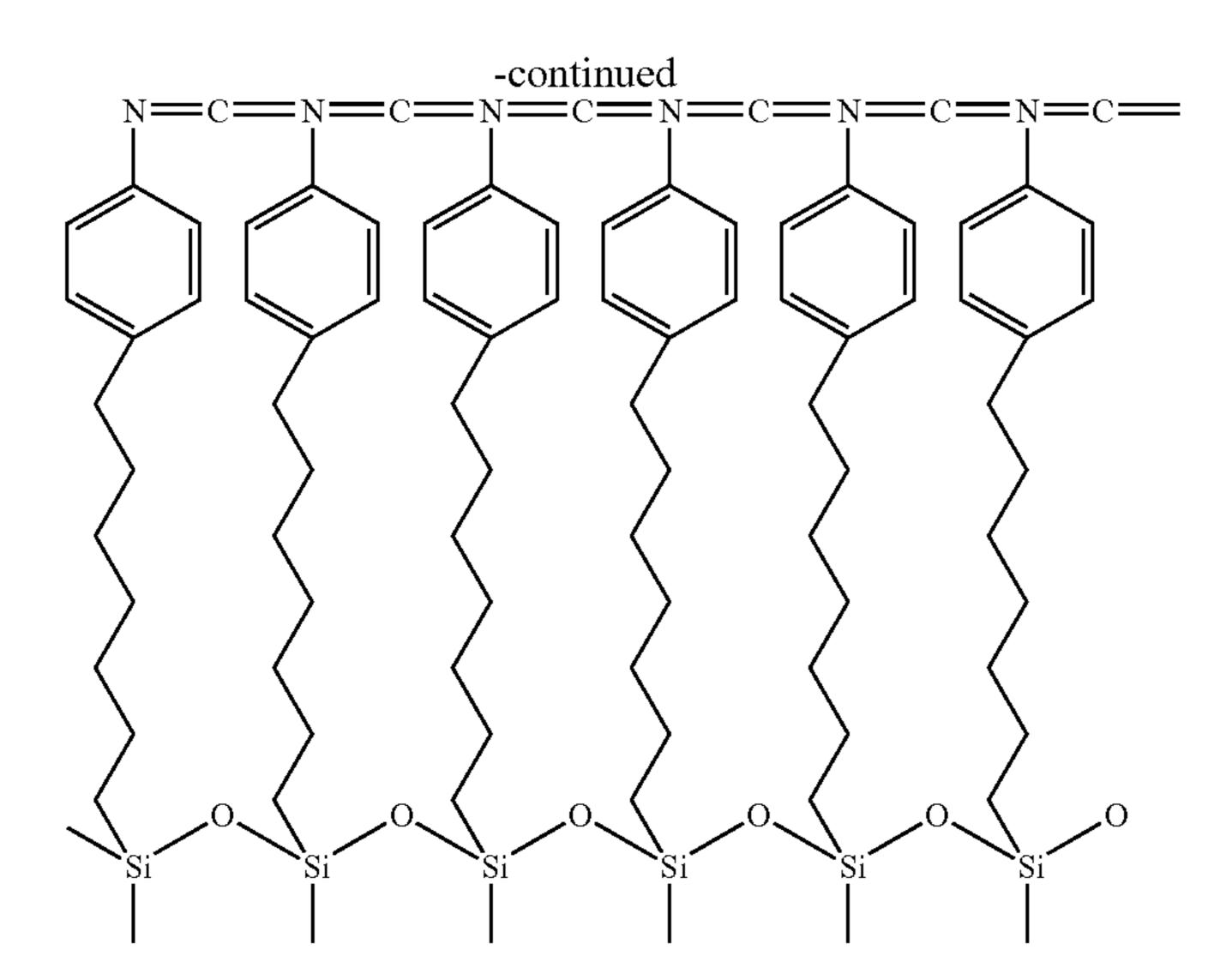
Example 2, above, illustrates a thermally induced polymerization of an end-cap functionality of isonitrile in a bifunctional molecule to form a polymerized SAM, which may be disposed on a substrate surface located between the source and drain electrodes of a field-effect transistor. This polymerized SAM includes an intramolecular charge trans-
