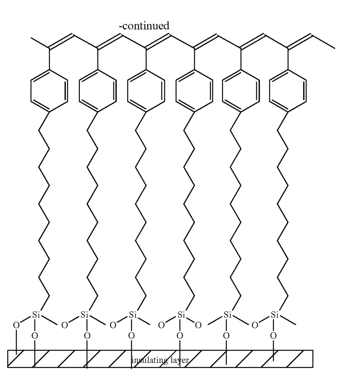
Example 3, above, illustrates a SAM of alkylphenylacetylene on an oxide insulating layer that has been polymerized by dipping in a solution of a catalyst, for example, a Ziegler catalyst, to form polyphenylacetylene at the surface of a polymerized SAM, which may form an intramolecular charge transport pathway between source and drain electrodes of a field-effect transistor.
