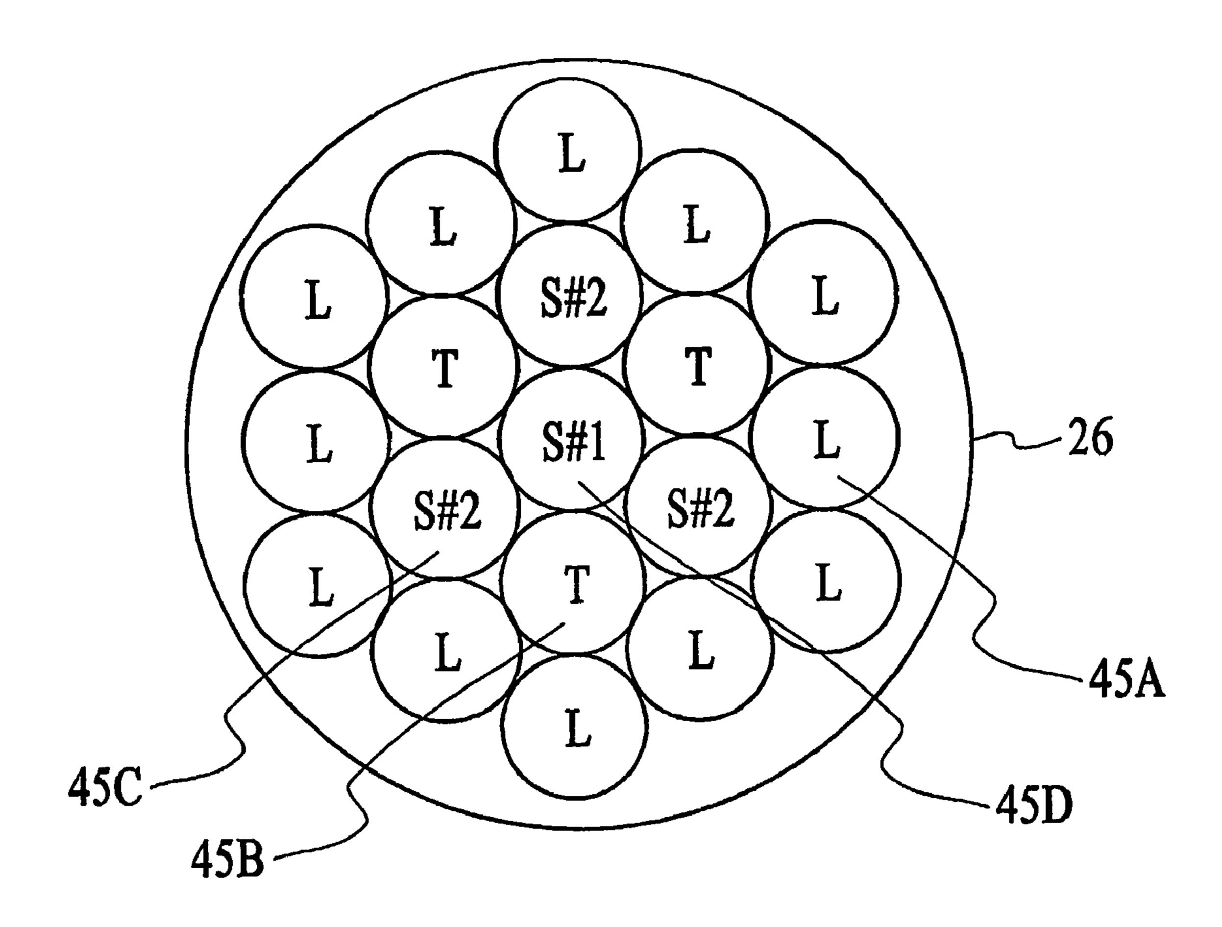
L = Light Source T = Topology S#1 = Spectrometer #1 Fiber S#2 = Spectrometer #2 Fibers
