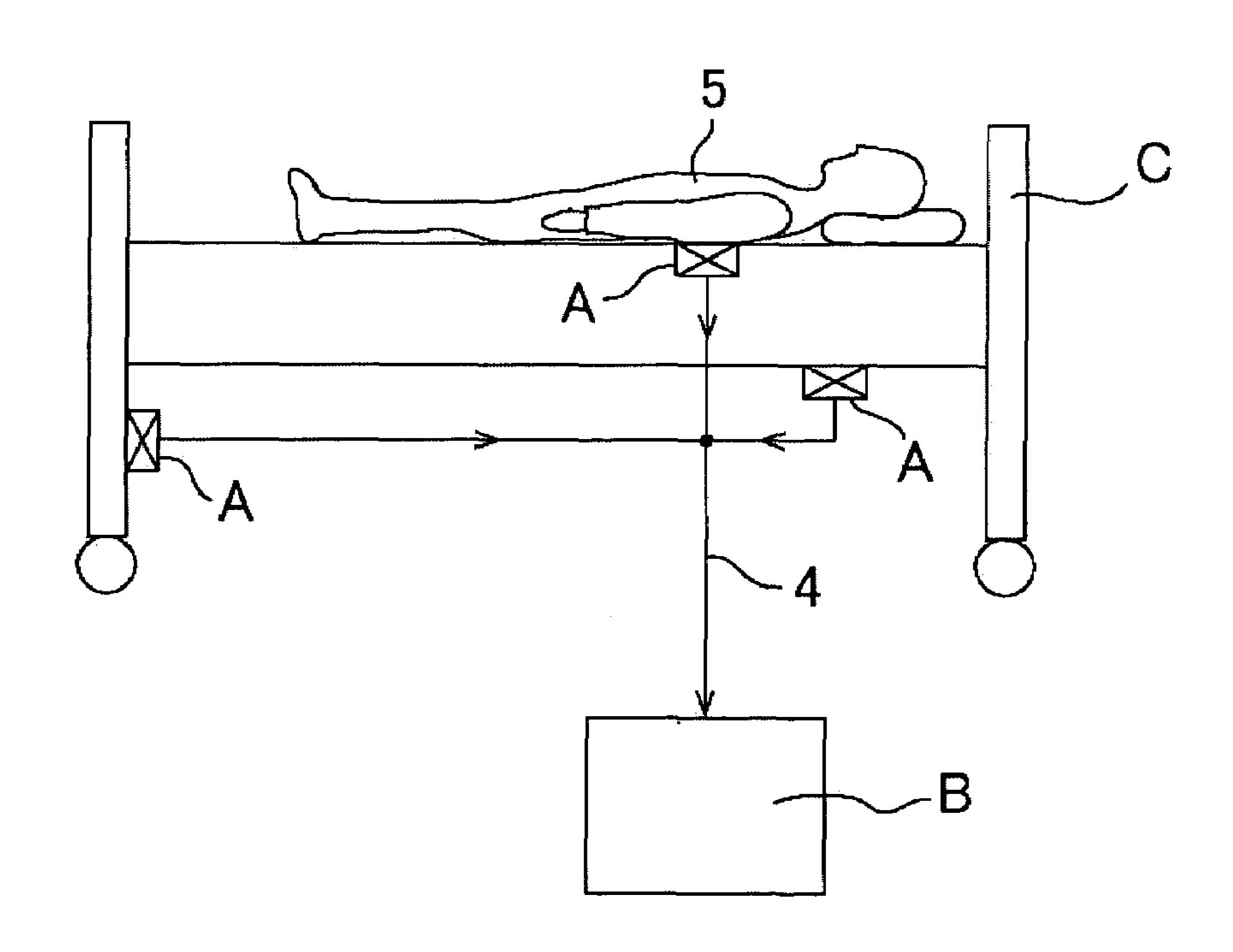
STATUS DISCRIMINATING APPARATUS OF HUMAN, ANIMAL, MACHINE OR THE LIKE USING ULTRASONIC VIBRATION DETECTING SENSOR, AND STATUS DISCRIMINATING METHOD OF HUMAN, ANIMAL, MACHINE OR THE LIKE USING THE SAME
