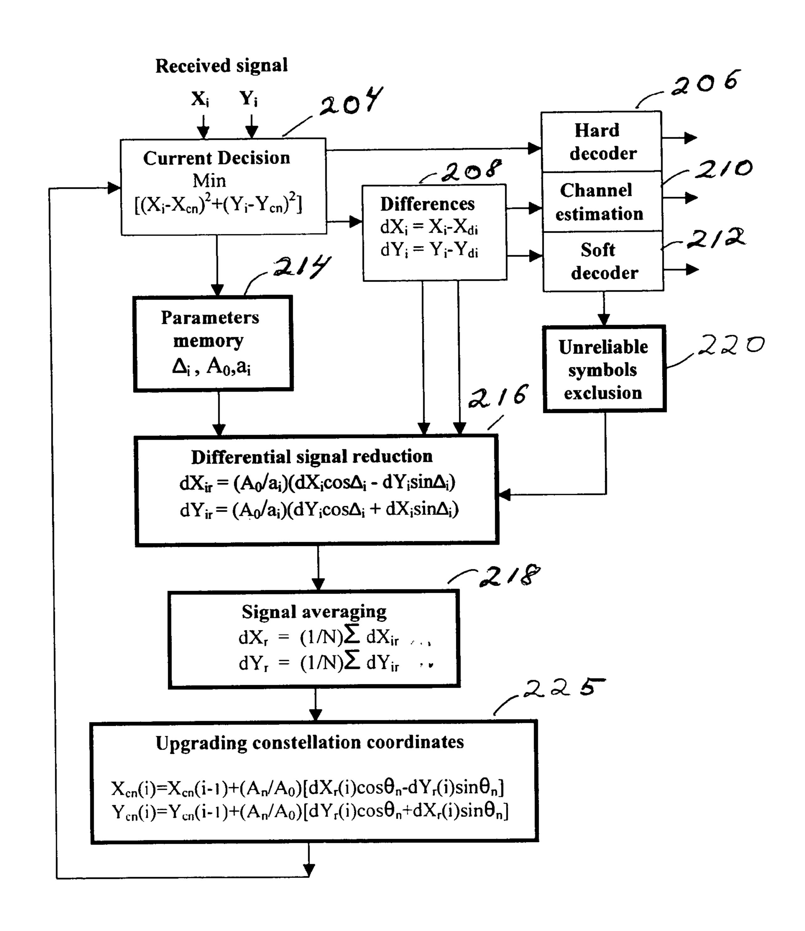
Fig.7 Correction of the received carriers in multicarrier system with correlated phase shifts, based on differential quadrature components of the received carriers
