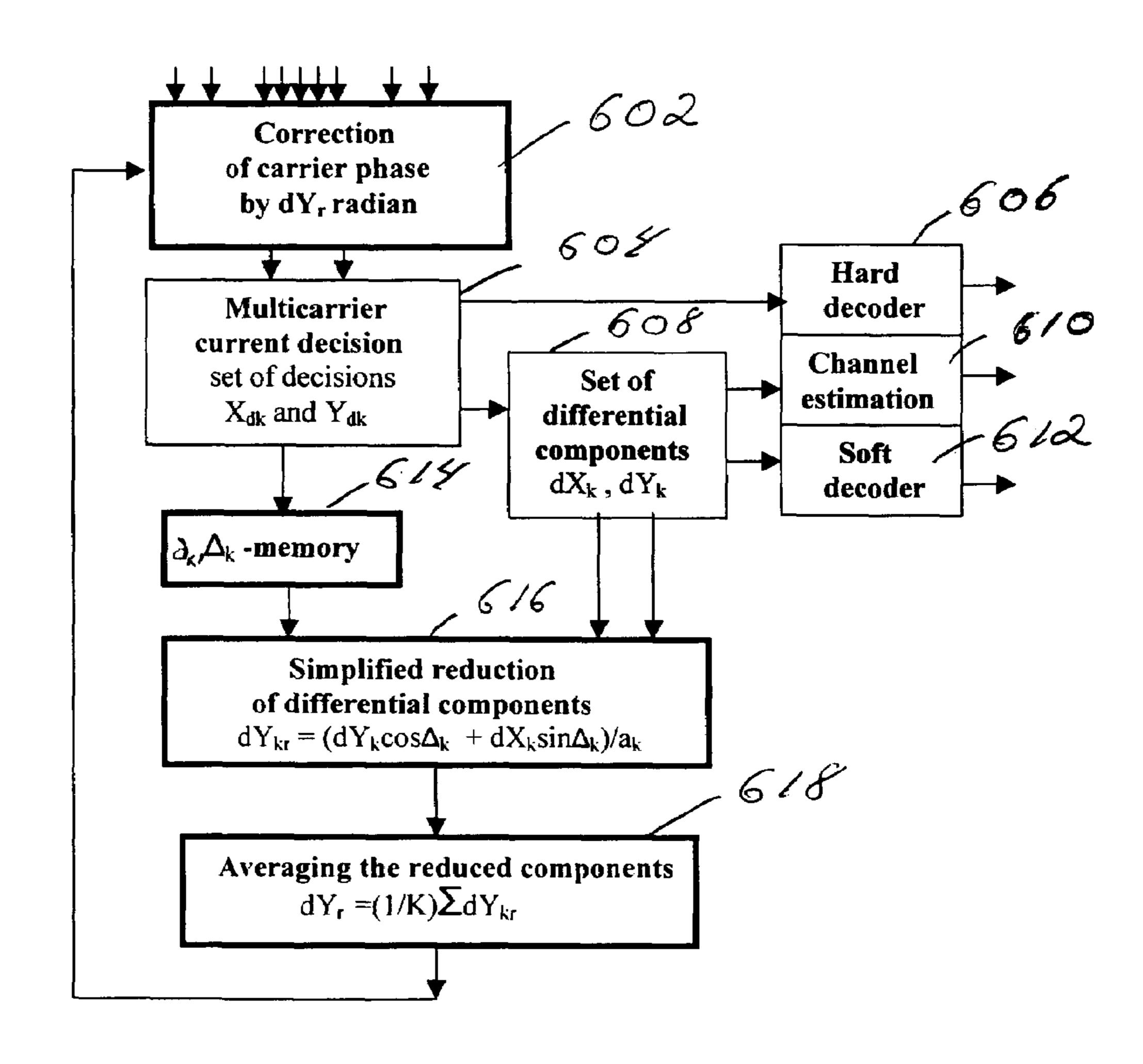
Fig. 11 Majority algorithm of carrier phase correction in multicarrier systems, based on the quadrature differential components.
