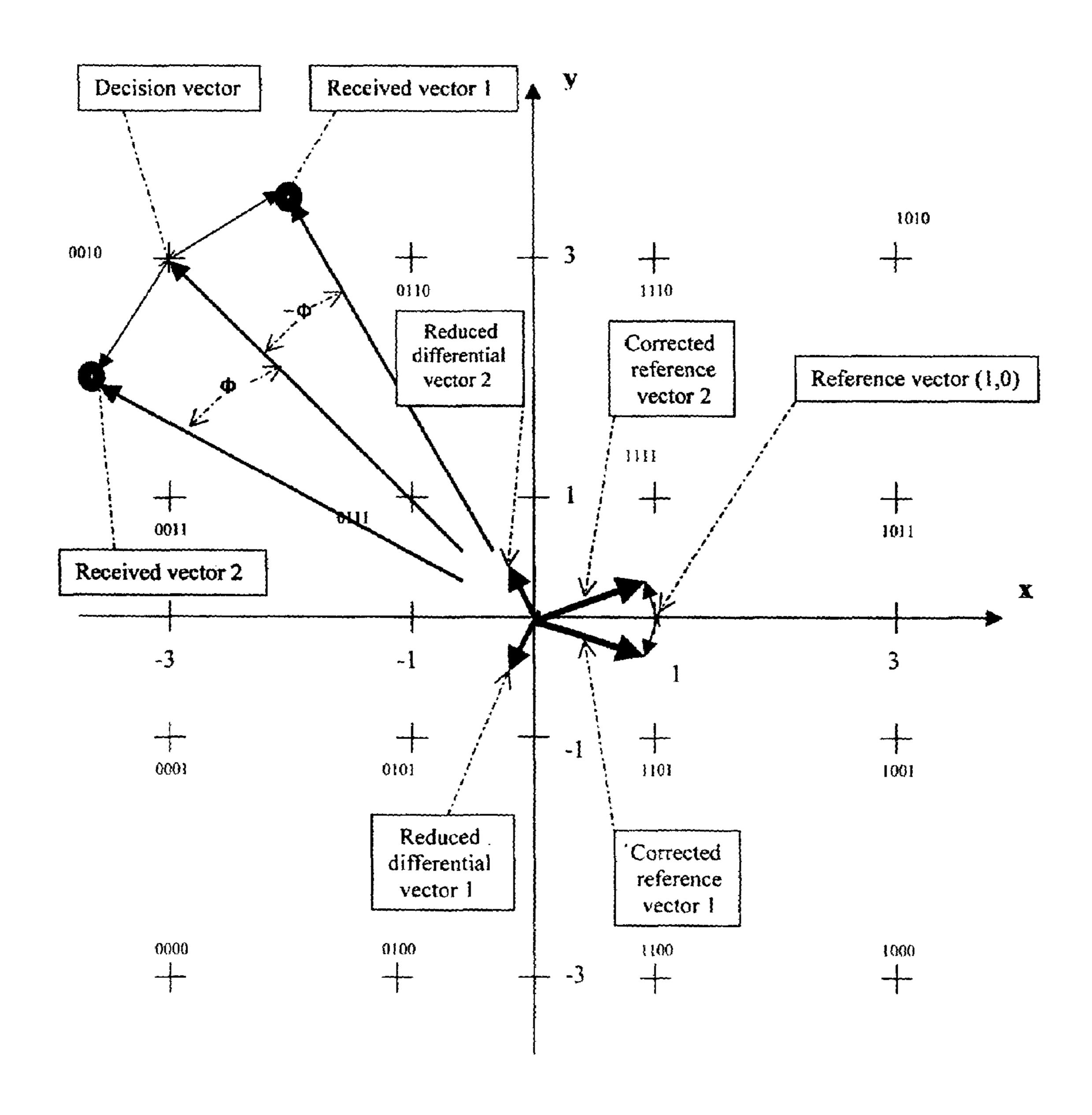
Fig. 10 Simplified carrier phase correction in multicarrier systems, based on the quadrature differential components.
