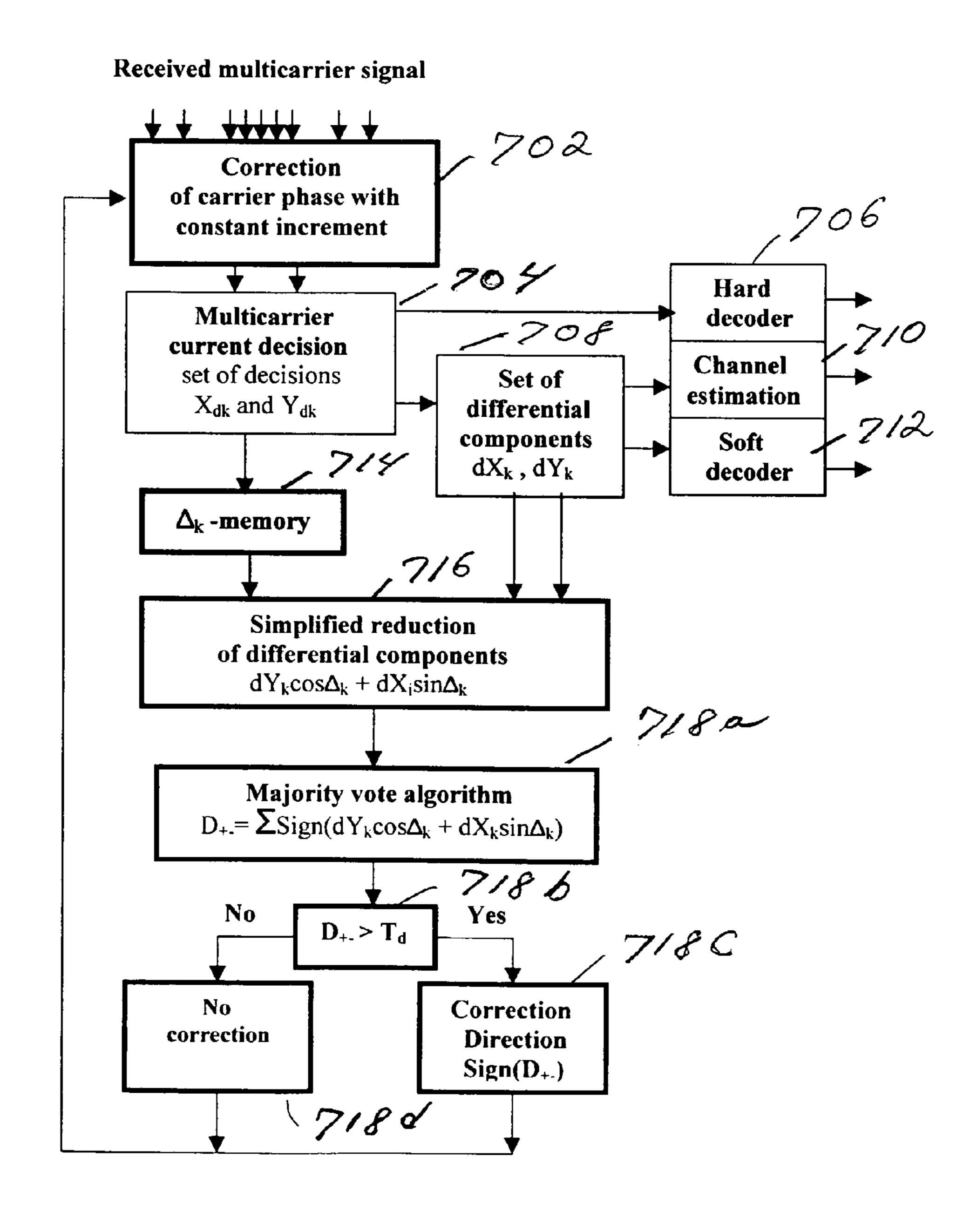
Fig. 12 Per-carrier adaptive equalizer, based on estimates of differential quadrature components.
