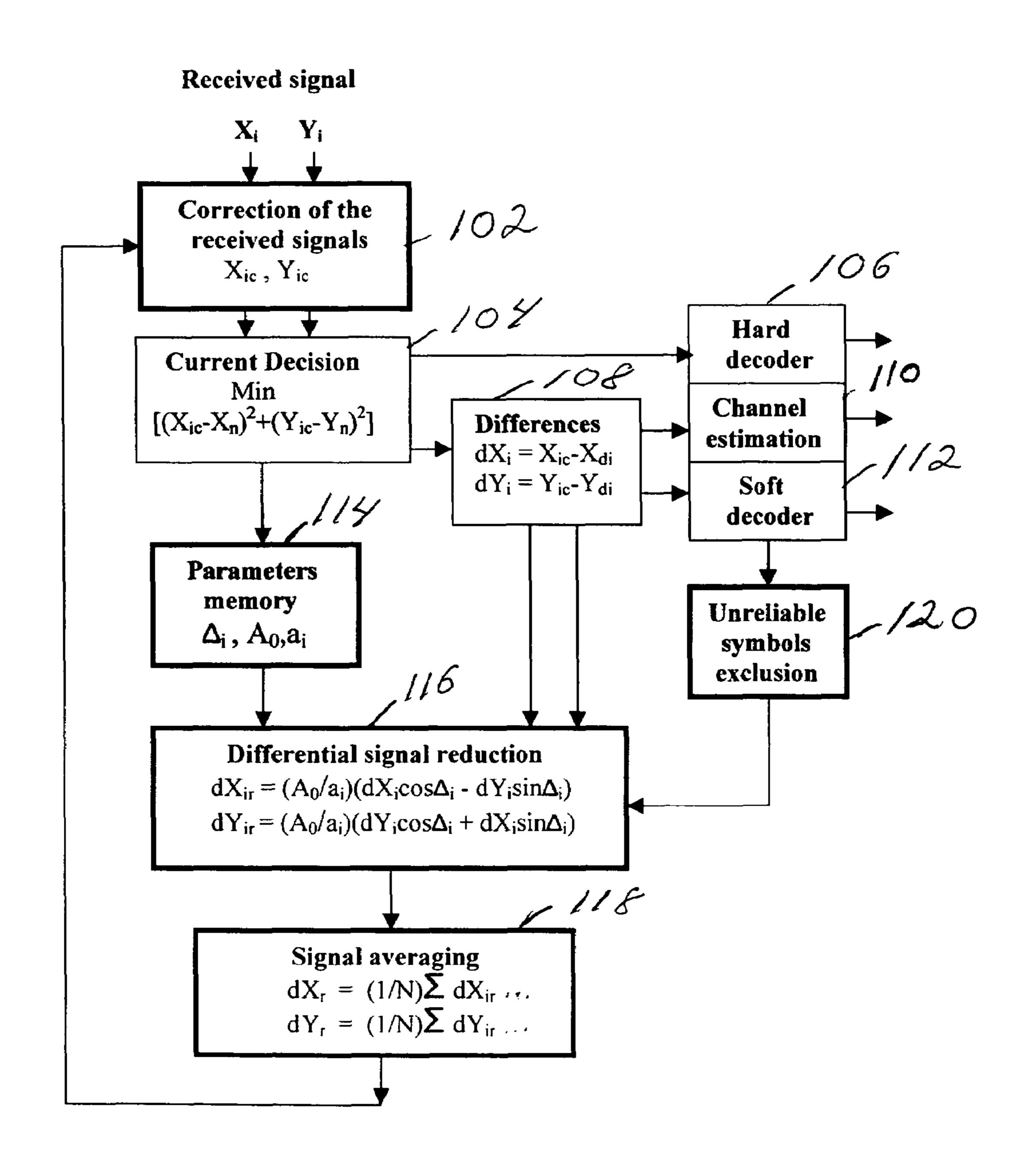
Fig.6 Correction of the constellation point coordinates, based on reduction and averaging differential quadrature components of the received signals
