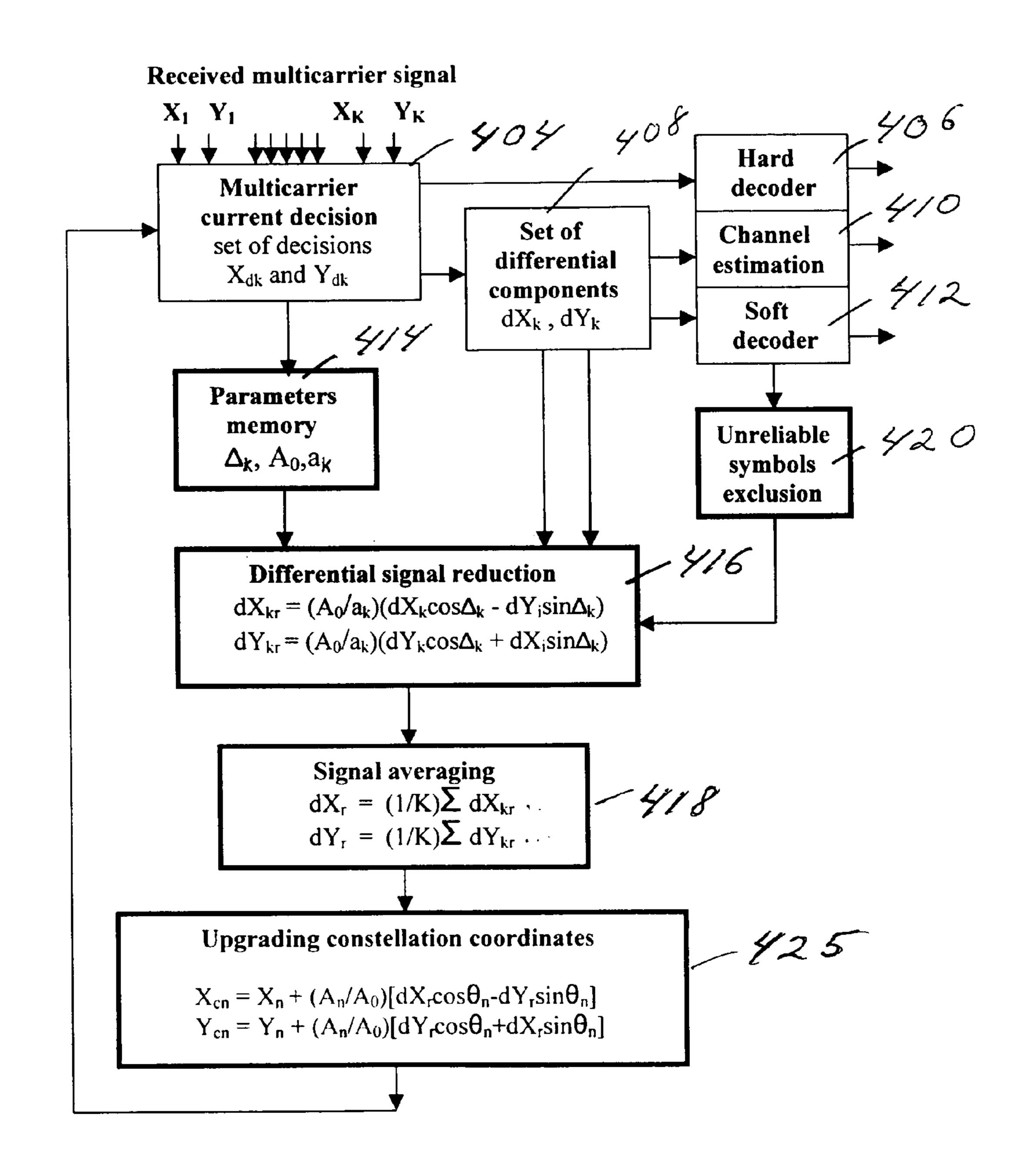
Fig. 9 Illustration to the simplified algorithms of phase correction.
