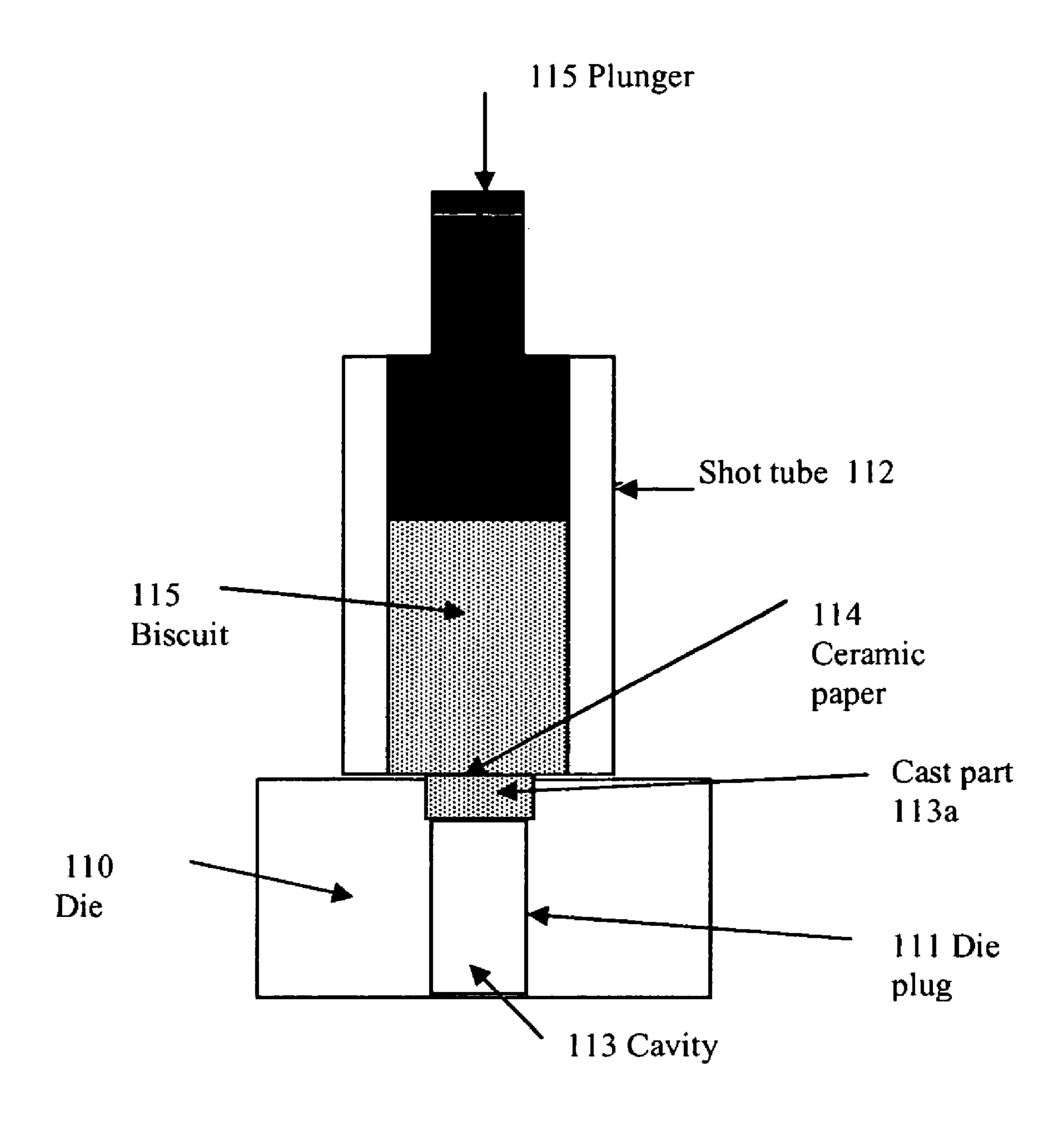
Figure 2- Schematic of the squeeze casting assembly
