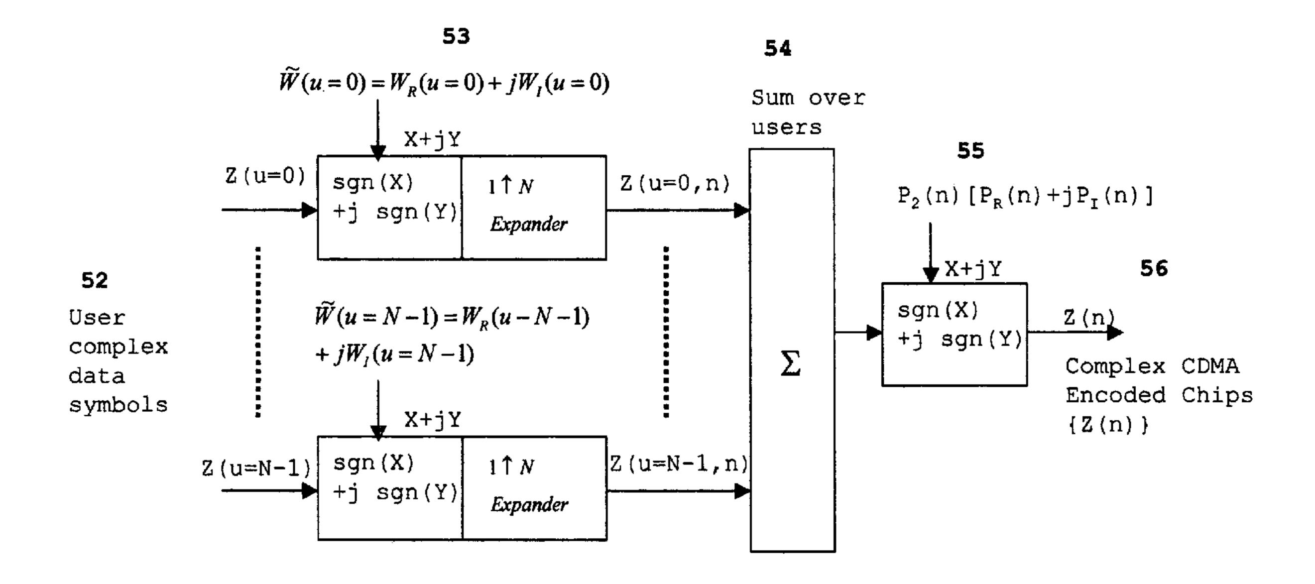
FIG. 1 CDMA Transmitter: Block Diagram
