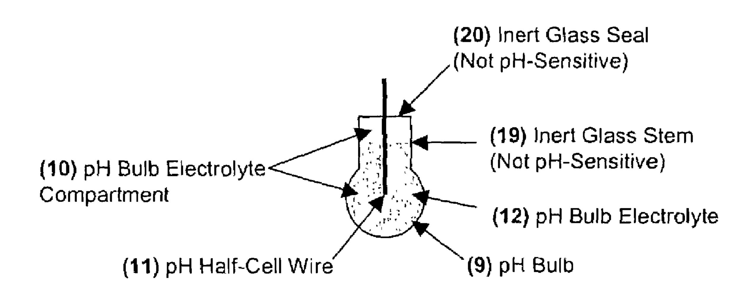
FIGURE 3 Combination pH Electrode with Alternative Venting System
