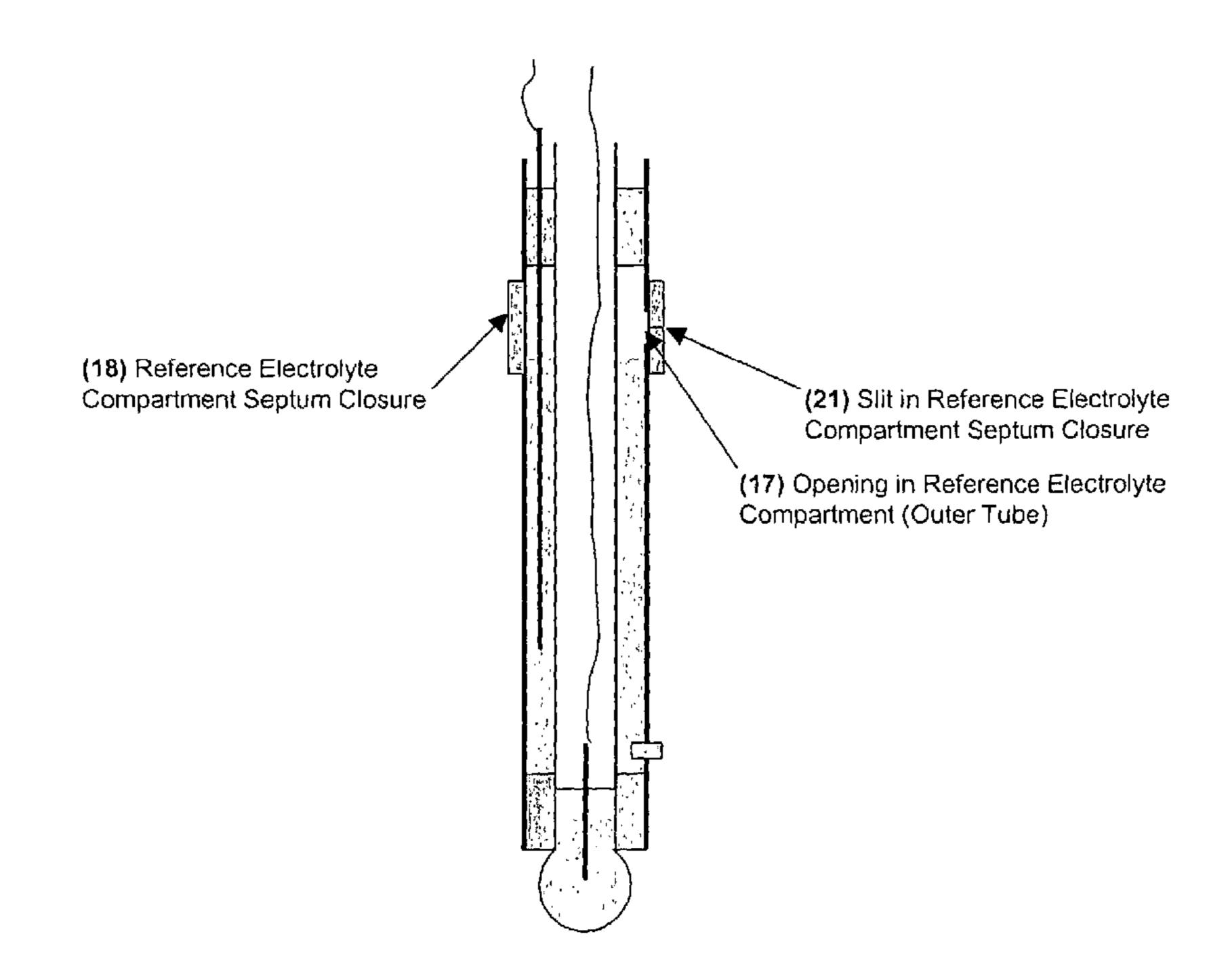
FIGURE 1 Basic Elements of Combination pH Electrode
