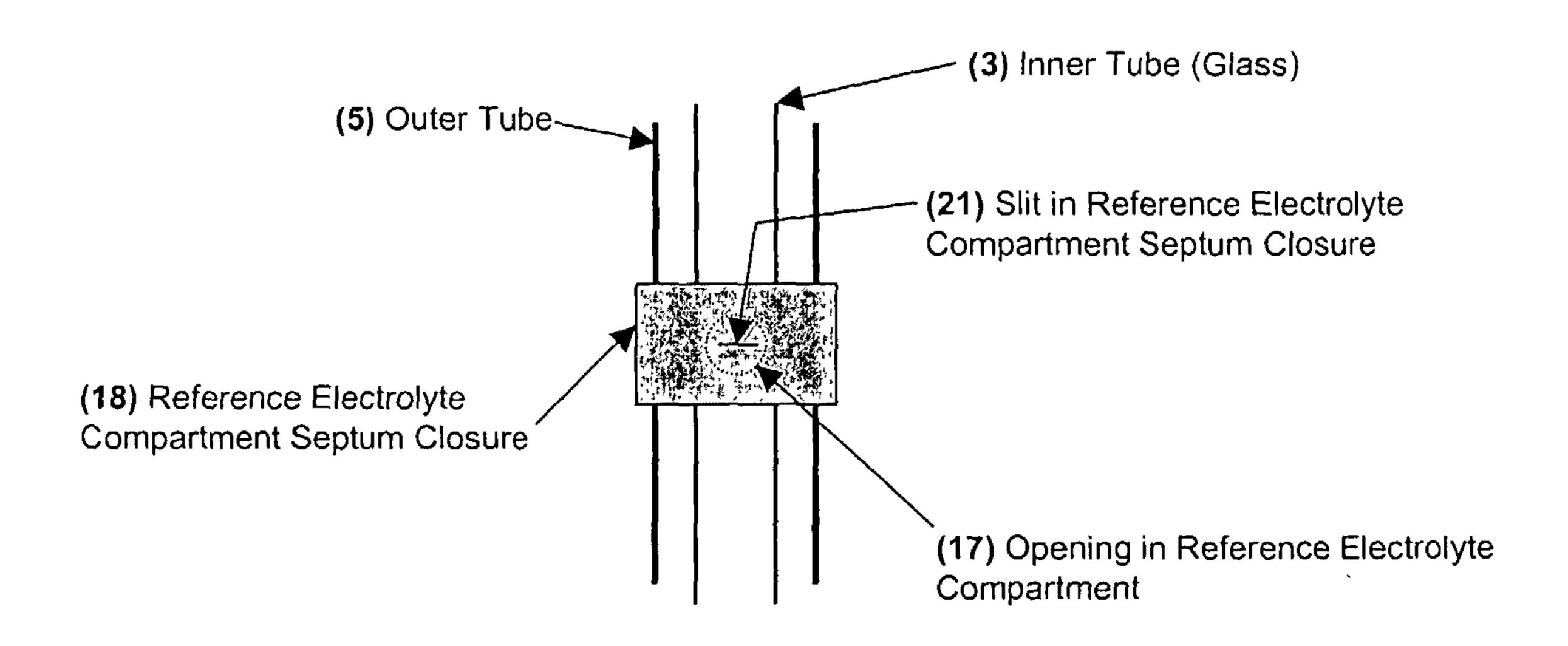
FIGURE 5 Combination pH Electrode and Storage Sleeve
