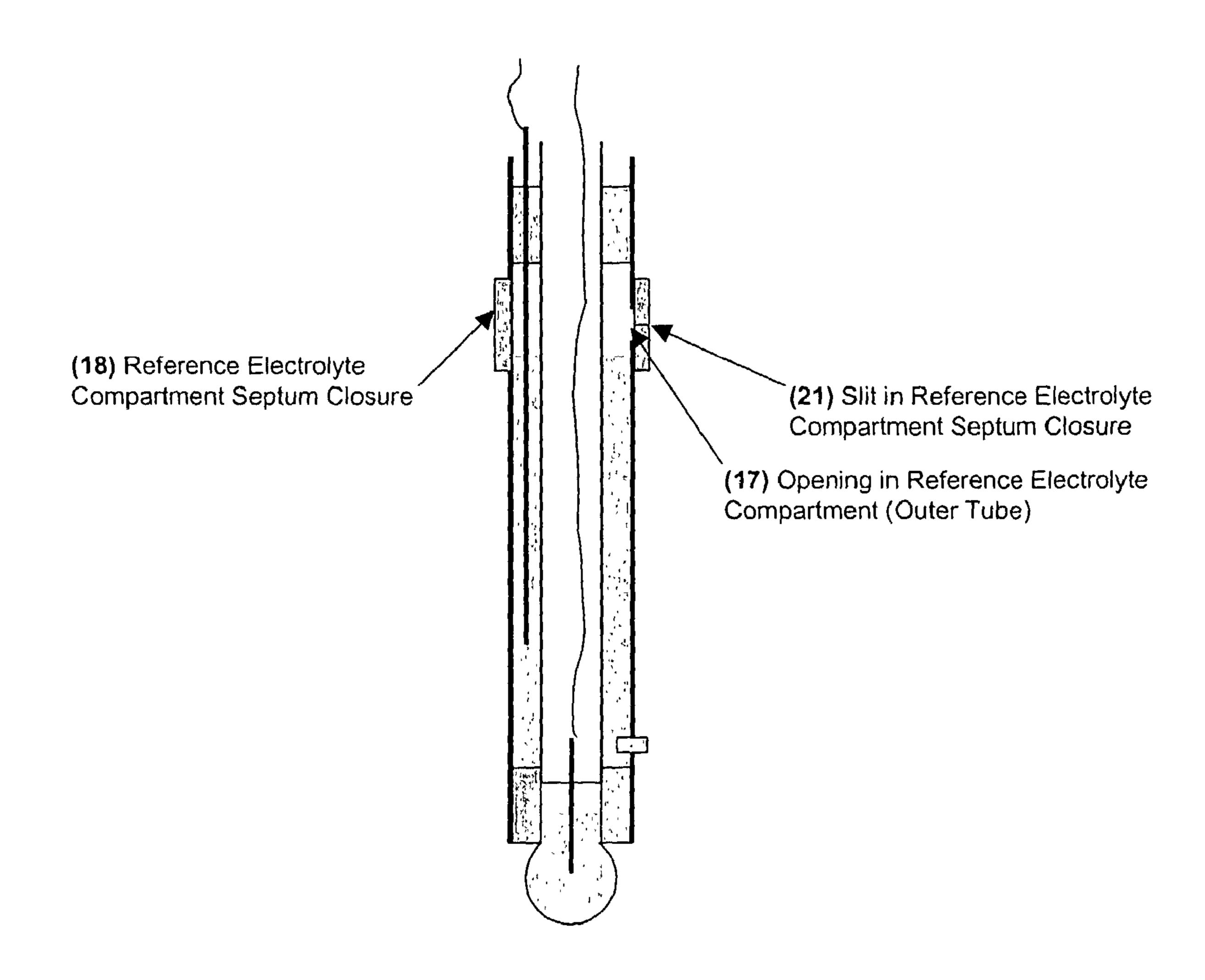
FIGURE 4 Front View of Septum Closure with Alternative Venting system
