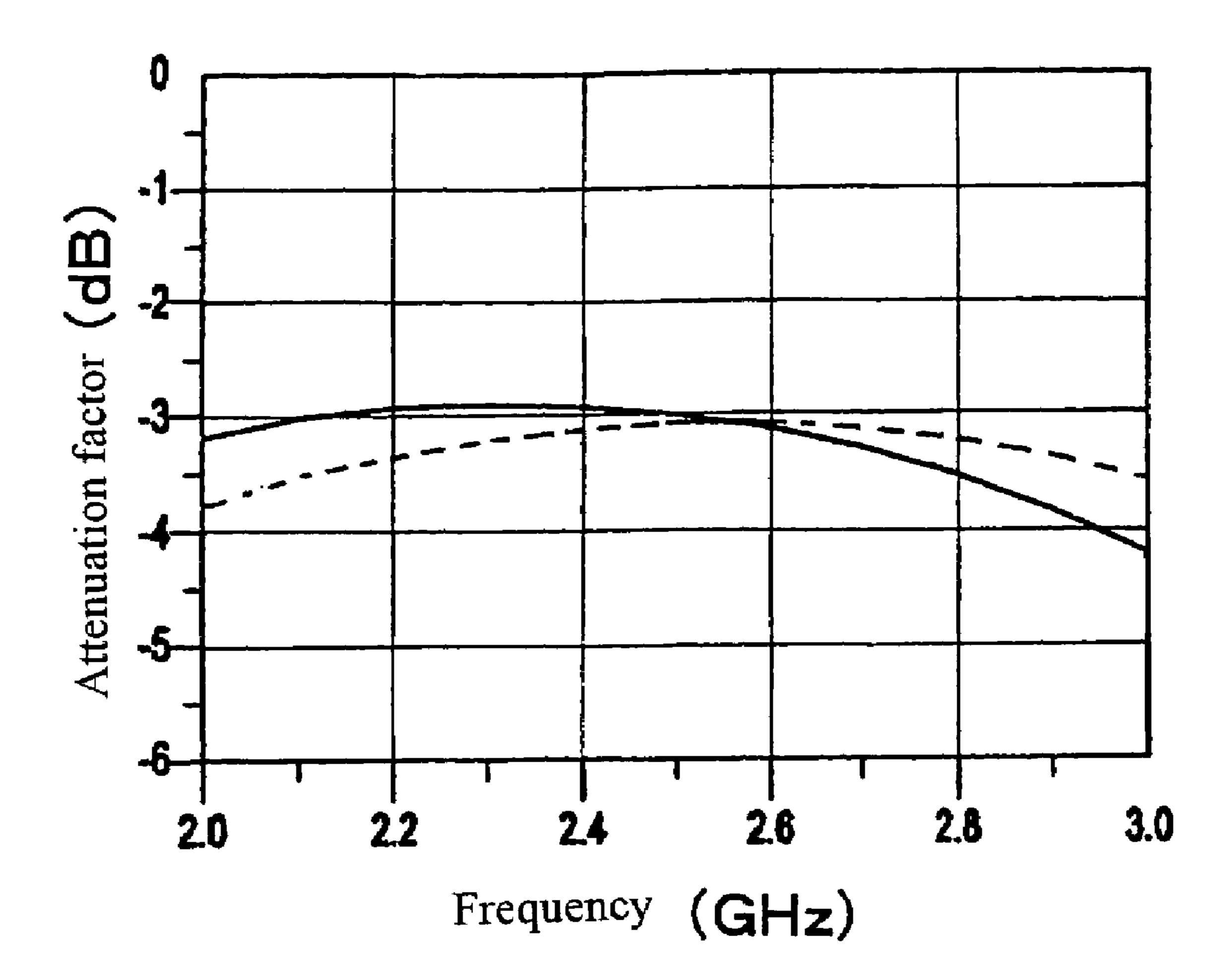
Permeability to output terminal 2 (S<sub>21</sub>)
