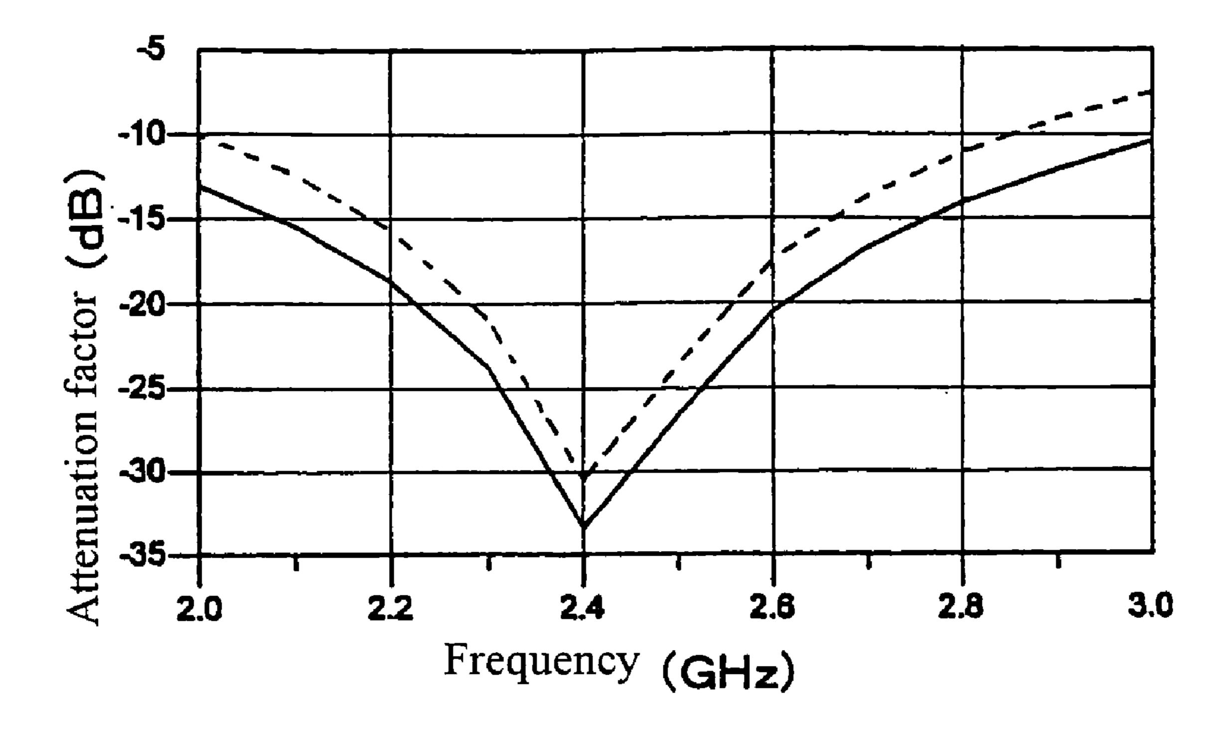
Reflection that occurs when differential amplitude is provided to output terminal 2 and output terminal 3
