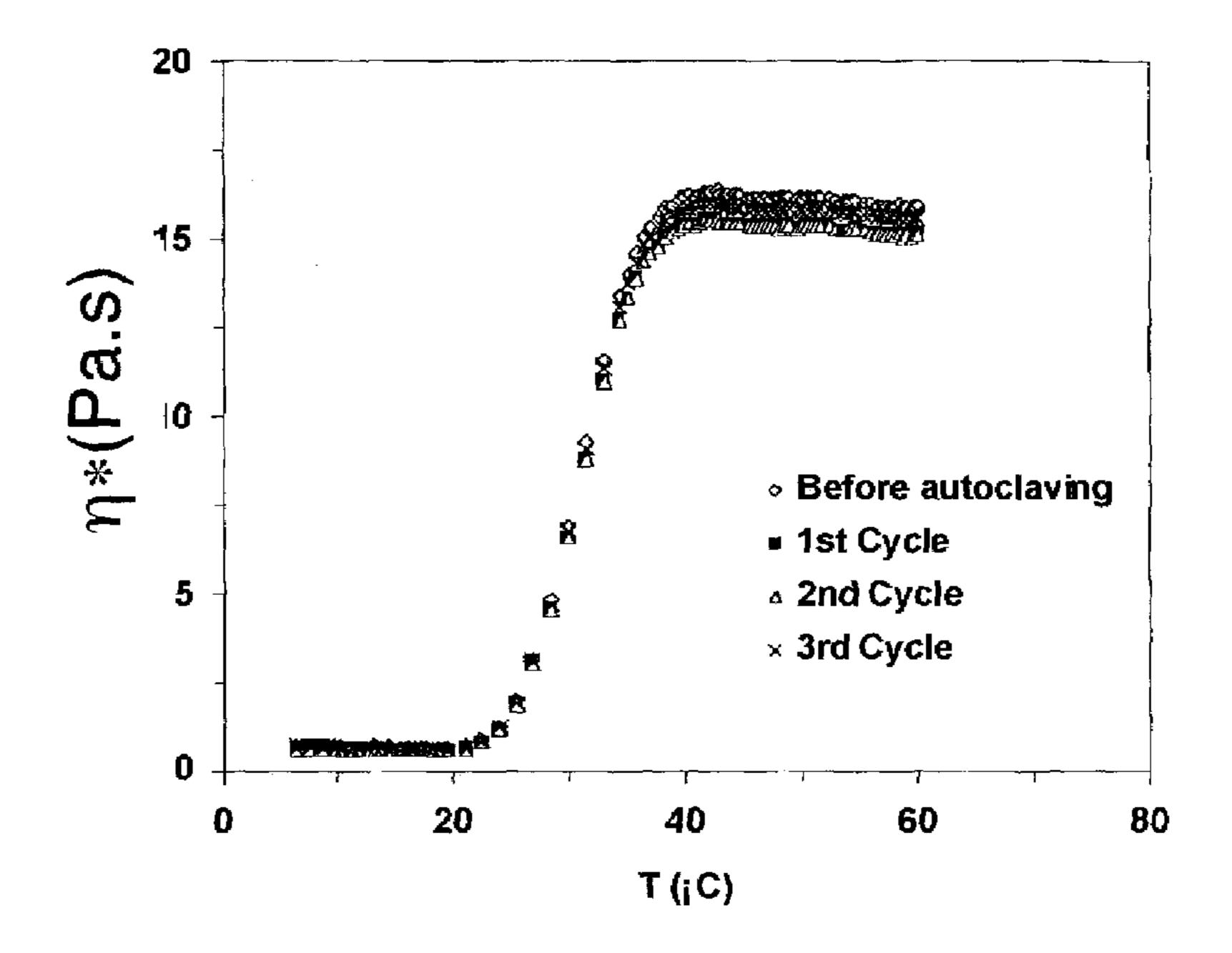
Rheological testing of "stabilized" 2 w/v% aqueous solution of Pluronic-PAA (pH
