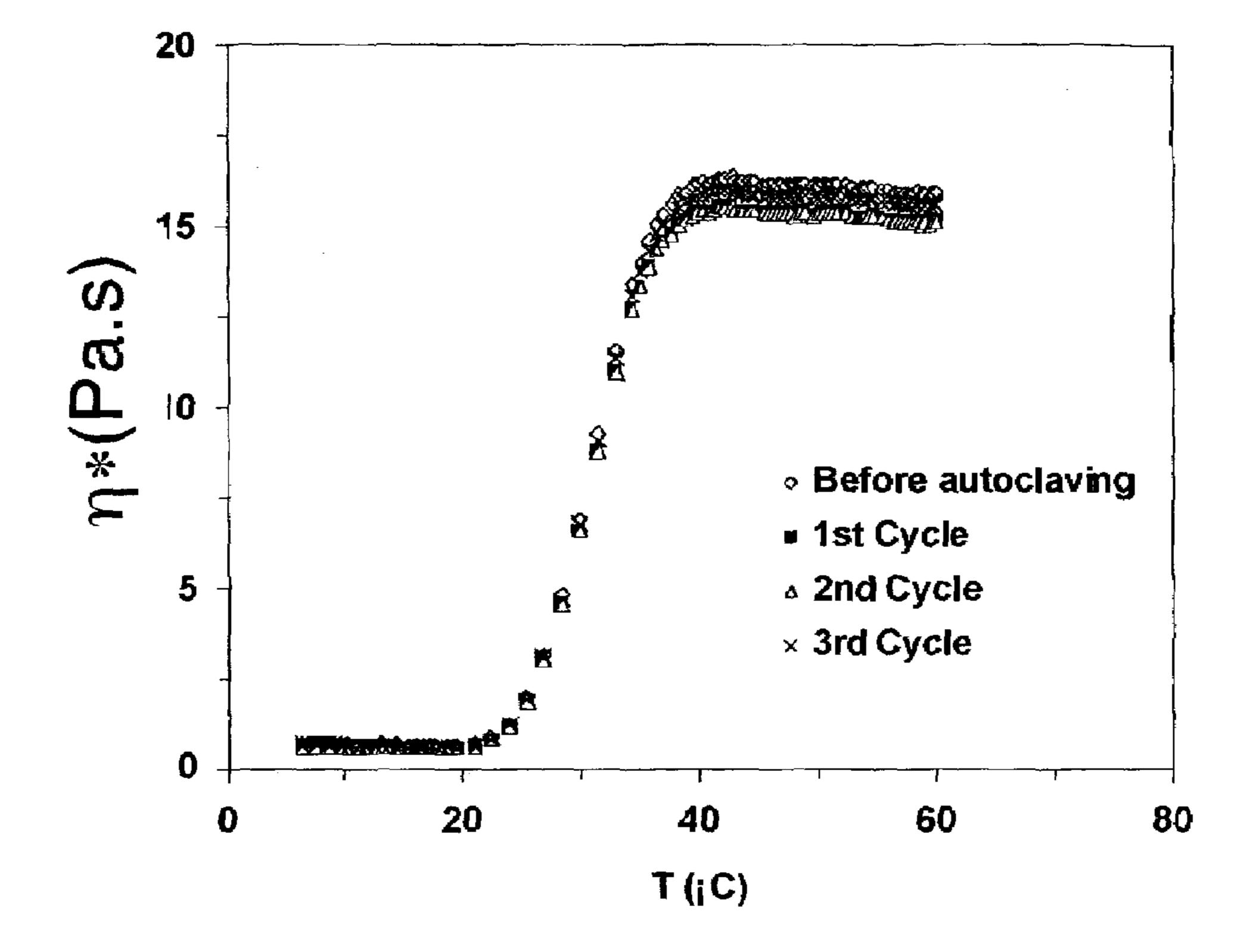
Fig.2. Rheological testing of "stabilized" 2 w/v% aqueous solution of Pluronic-PAA (pH 7.0) before autoclaving and after each consecutive cycle of autoclaving. Frequency of oscillatory shear 6.28 rad/s, strain 1.7%.
