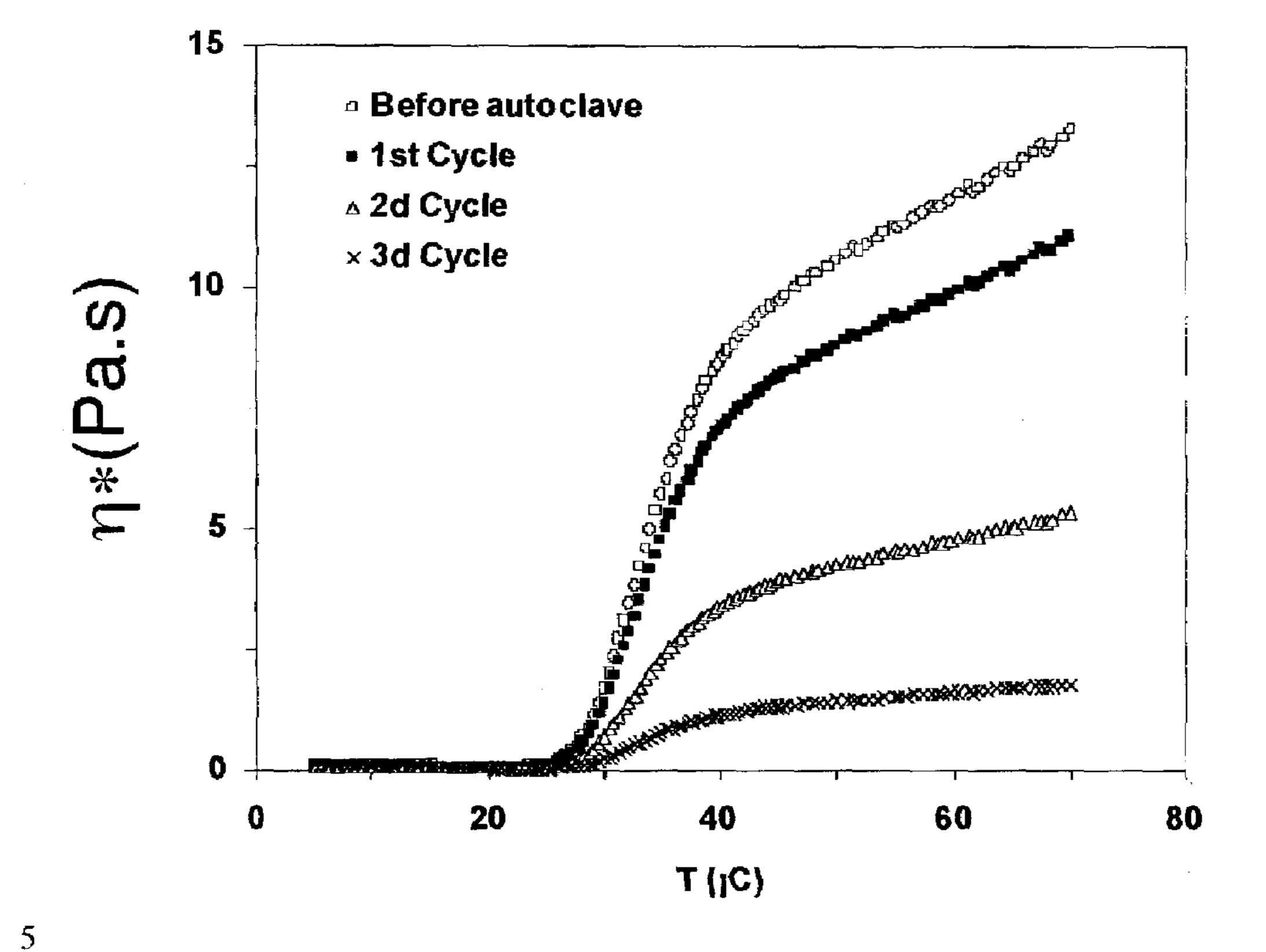
Fig.1. Rheological testing of "unstabilized" 2 w/v% aqueous solution of Pluronic-PAA (pH 7.0) before autoclaving and after each consecutive cycle of autoclaving.
