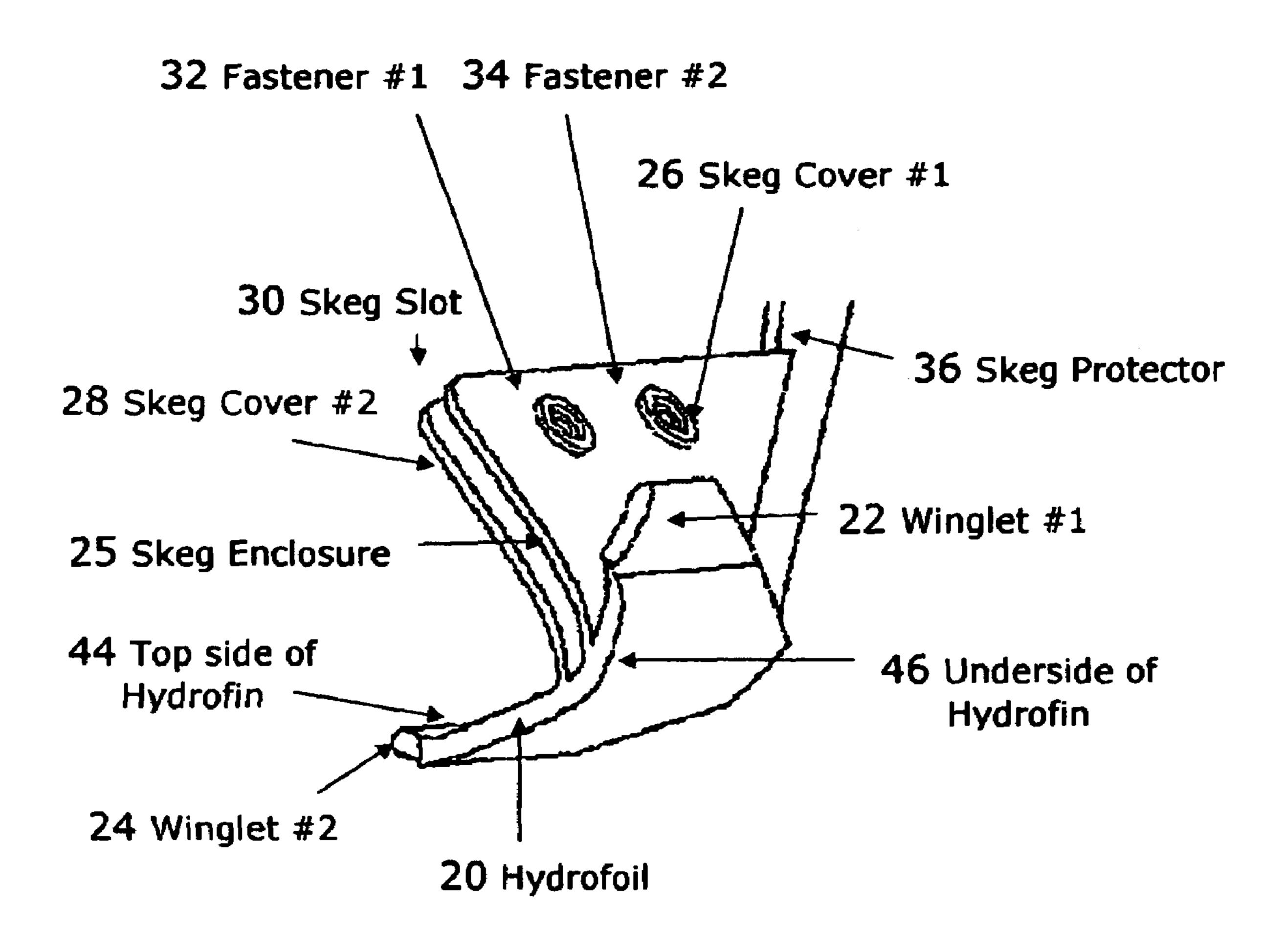
Figure 2. Hydrofoil with Skeg Enclosure
