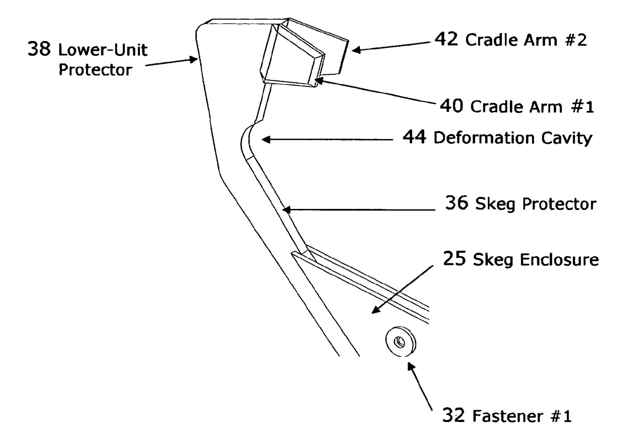
Figure 3. Skeg Enclosure with Skeg Protector and Lower-Unit Protector
