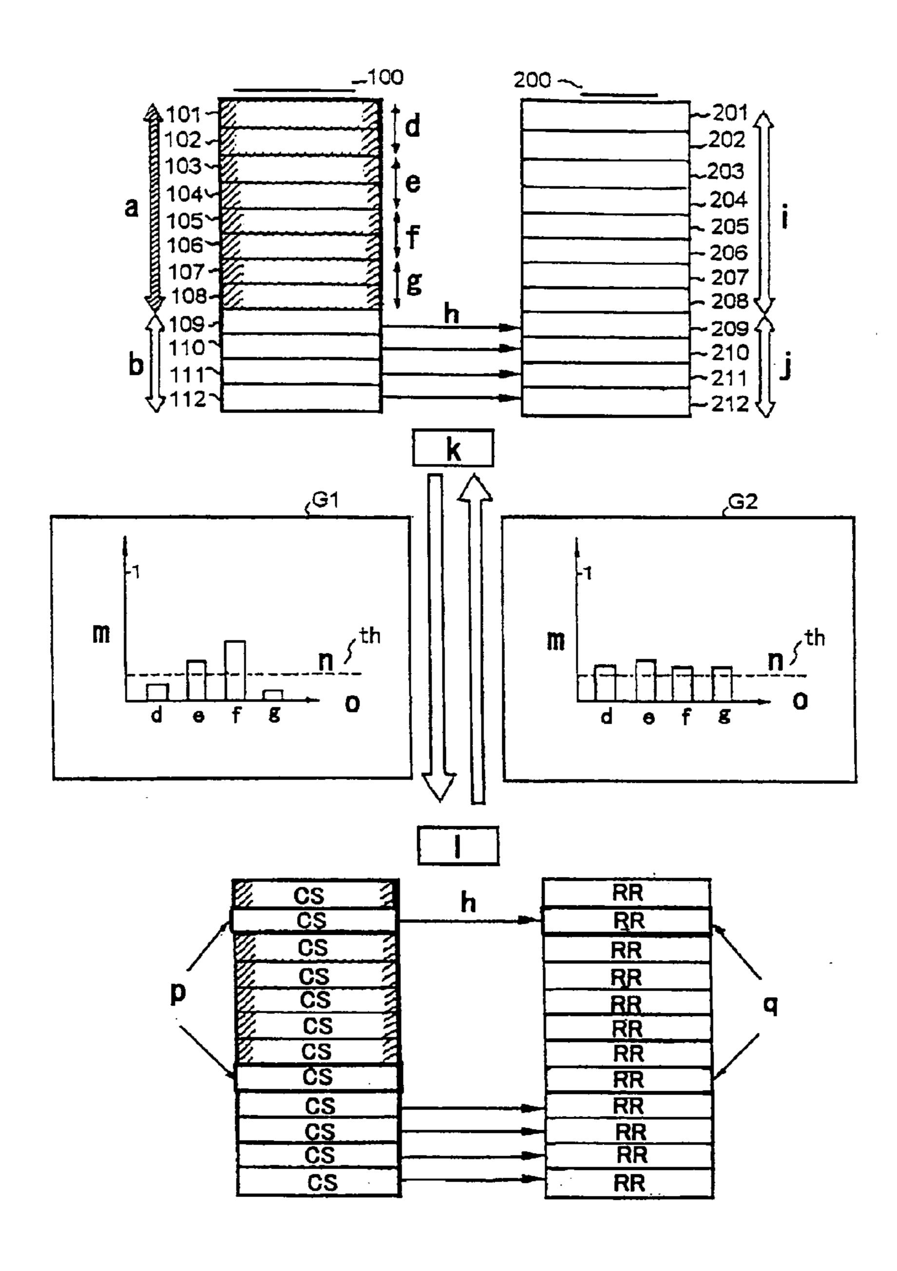
100: PATH DETECTOR 101-112: CORRELATOR SET 200: DECODER 201-212: RAKE RECEIVER
