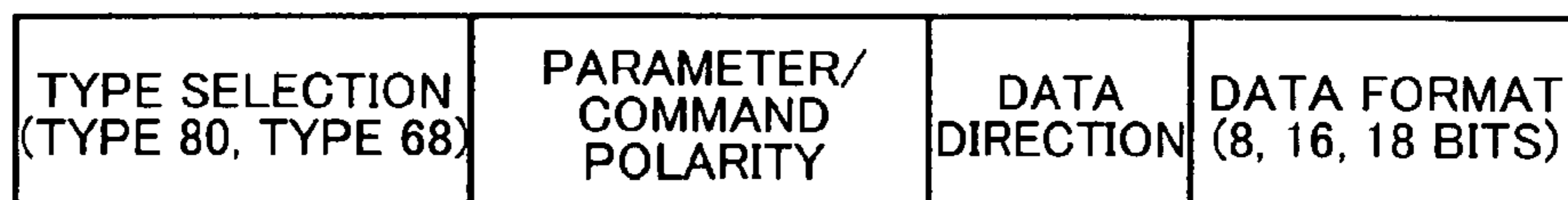
FIG. 14C MPU INTERFACE SETTING REGISTER
