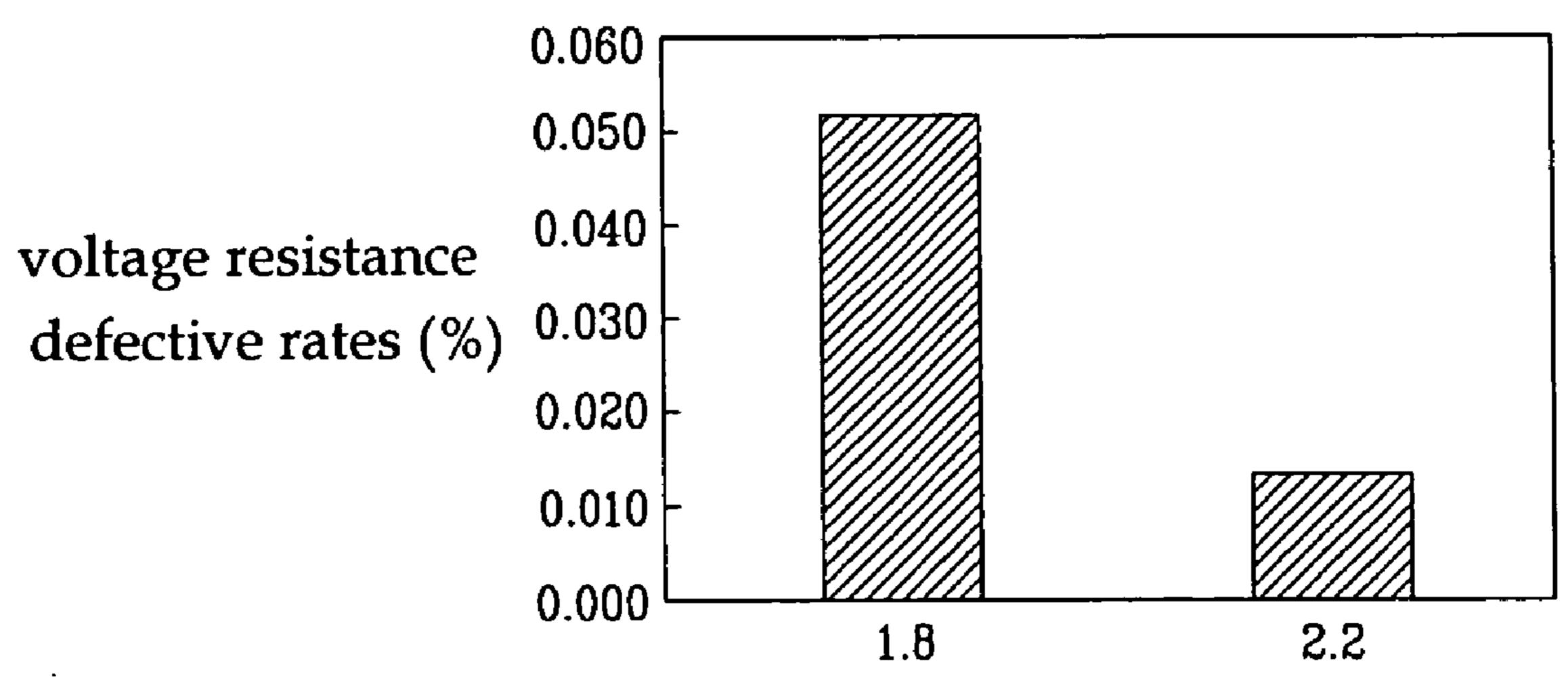
minimum gap between fourth electrode fifth electrode (mm)
