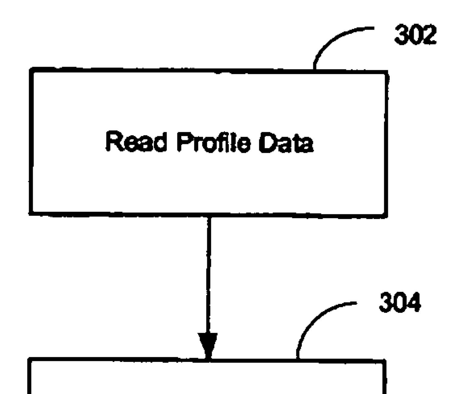
Transfer selected data from one or more mass storage devices into a cache memory, based on, at least in part, historical device access data comprised in Profile Data
