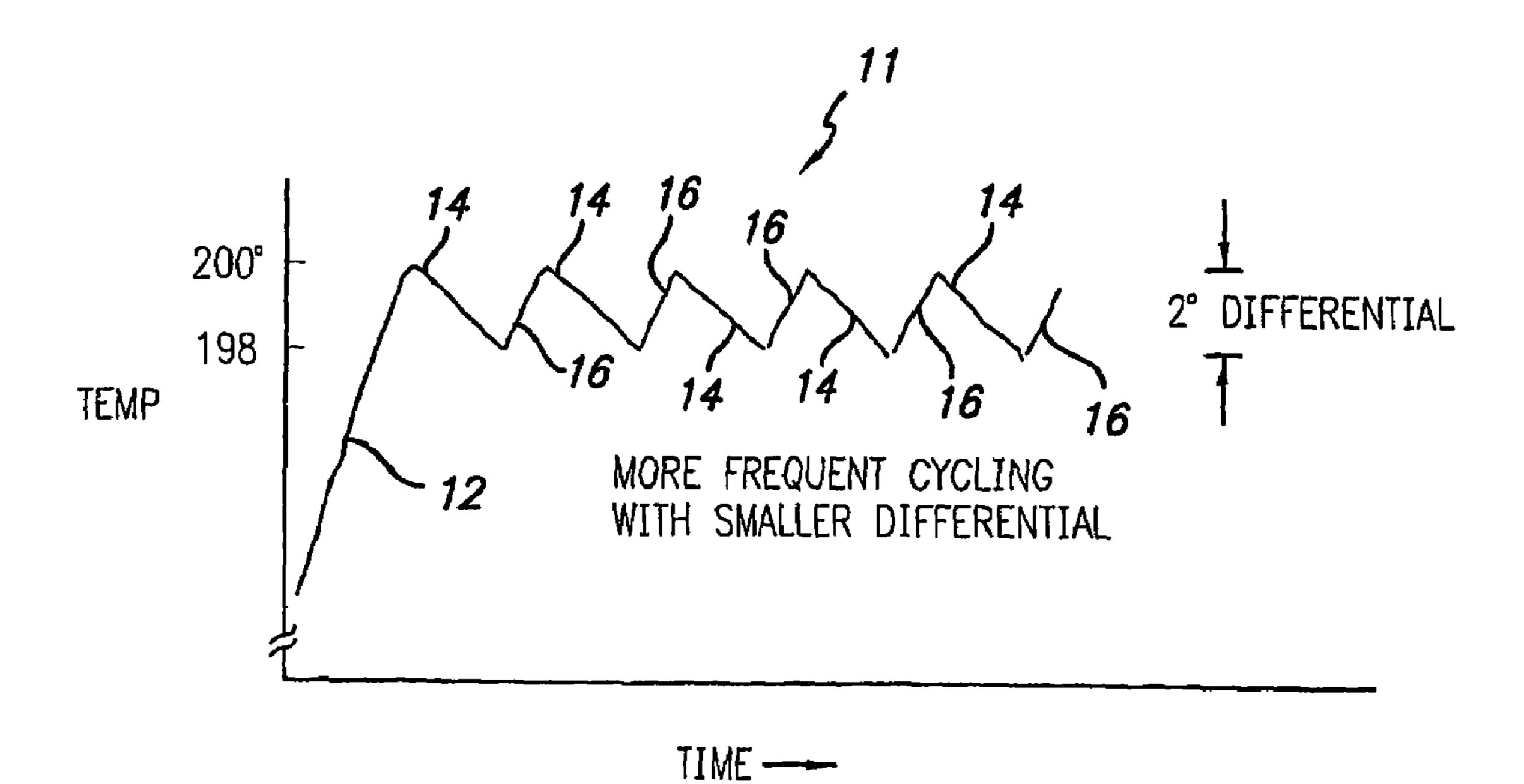
MECHANICALLY SWITCHED THERMOSTAT CHARACTERISTIC
