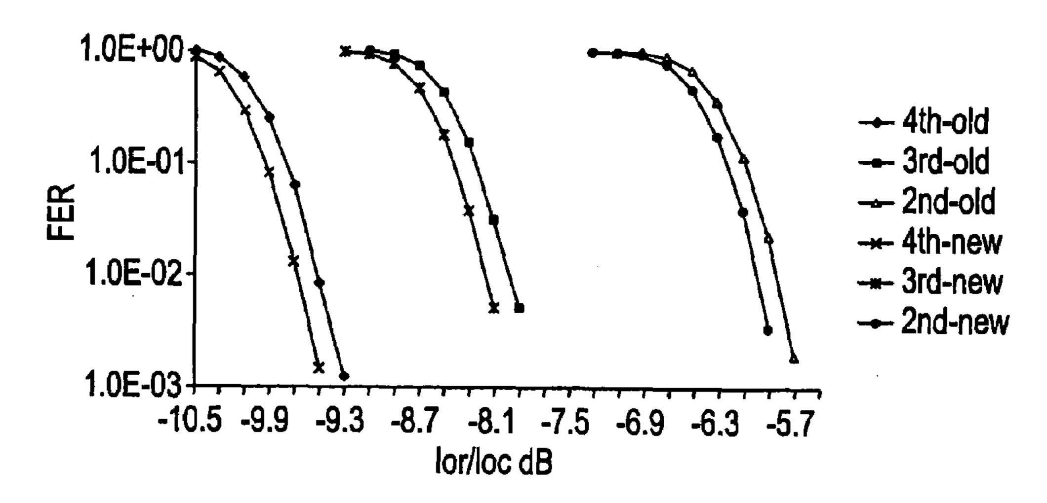
FER vs. lor/loc after 2, 3 and 4 transmissions. AWGN, Ec/lor = -1dB, 1 code 16QAM5/8.
