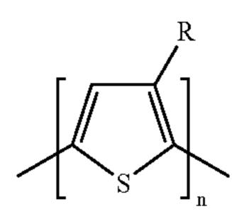
the polymer having a charge carrier mobility ( $\mu$ ) of at least about  $1\times10^{-2}$  cm<sup>2</sup>/Vs and an on/off ratio of at least about  $1\times10^3$ , and wherein n comprises from about 2 to about 10,000.
