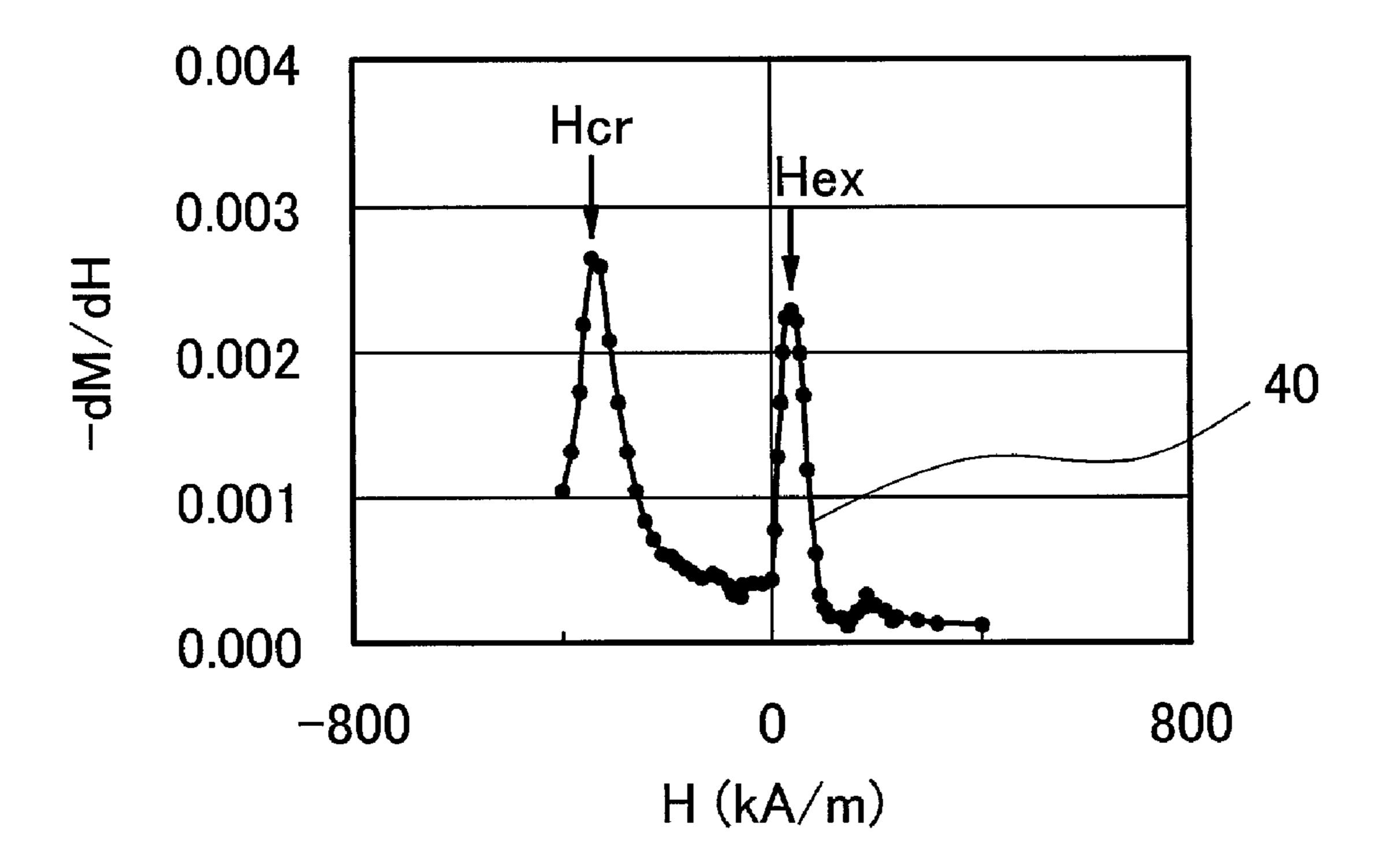
40···CURVE WHICH IS OBTAINED BY DIFFERENTIATING THE MAGNETIZATION M BY THE MAGNETIC FIELD H ON THE MAGNETIZATION CURVE 32
