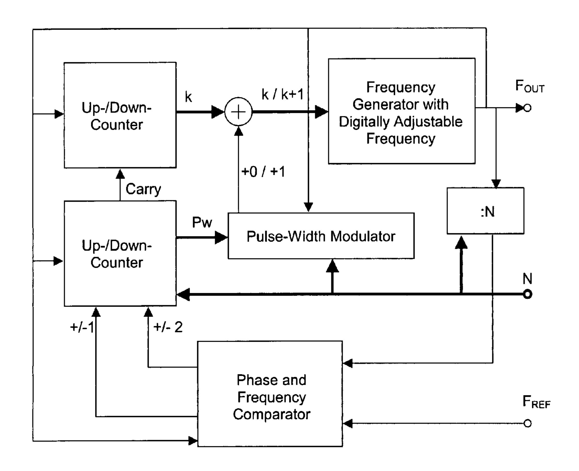
Fig. 2: Assembly of the Output Frequency with Pulses of two different Frequencies F<sub>1</sub> and F<sub>2</sub>
