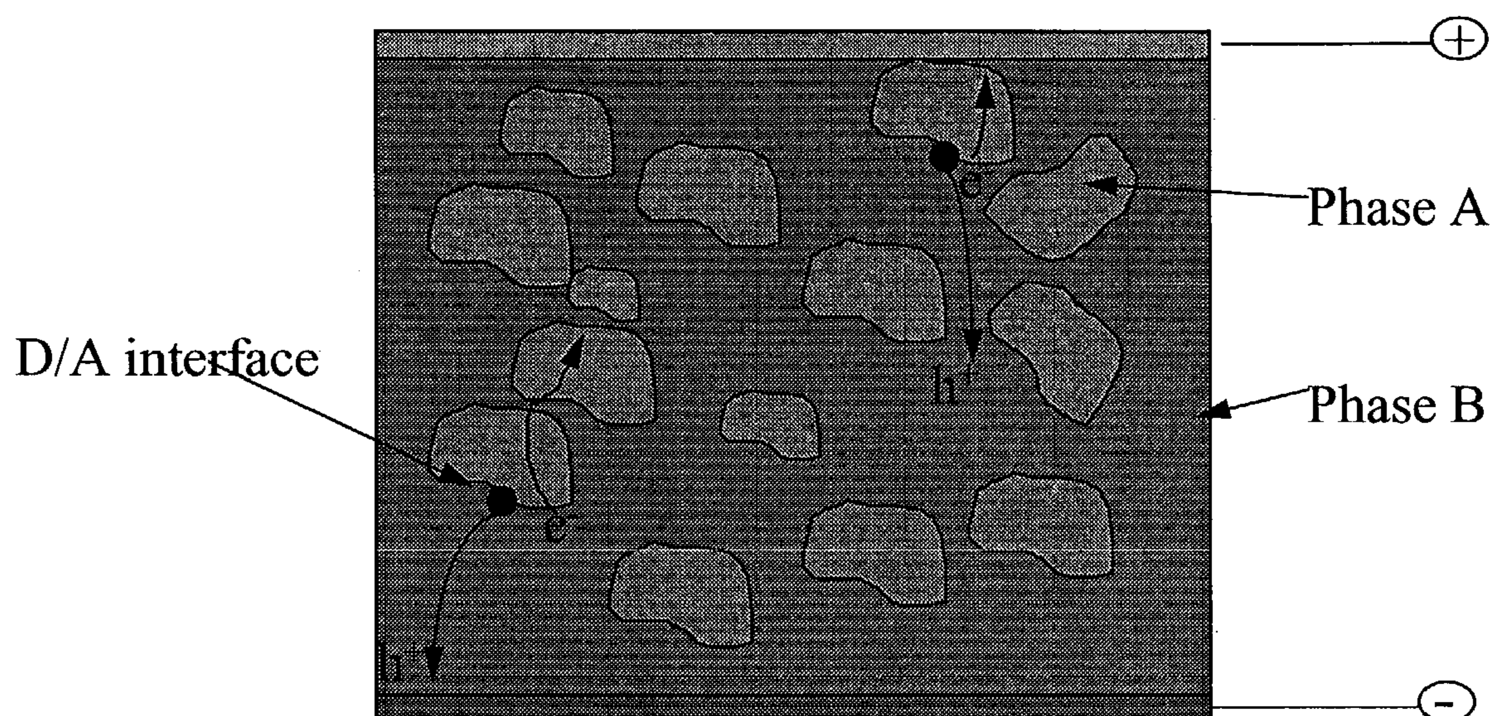
Fig.1 - seperated charges must be transported to their electrodes without touching the opposite phase to avoid recombination
