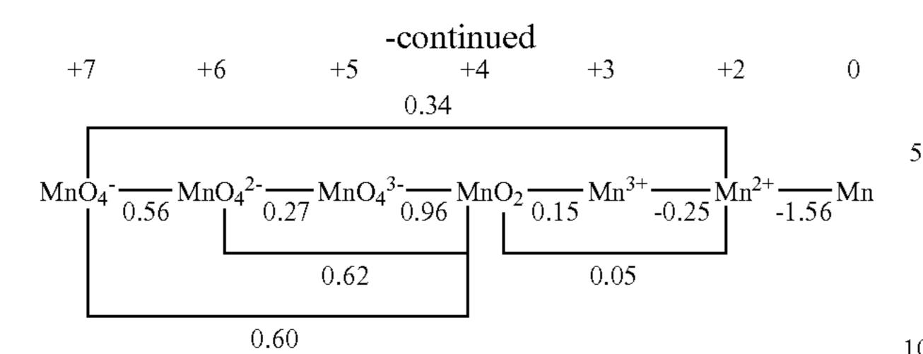
From consideration of the redox potential under basic conditions, the oxidation of low-covalent Mn(II) to Mn(IV) is much easier. Since the potential of MnO<sub>2</sub>/Mn(OH)<sub>2</sub> couple, E° MnO<sub>2</sub>/Mn(OH)<sub>2</sub>=-0.05V, is lower than that of O<sub>2</sub>/OH— couple, E°=0.401V, Mn(OH)<sub>2</sub> can be easily oxidized than, for example, Mn(OH)<sub>4</sub>, by molecular oxygen in air to form oxo compounds, as follows:
