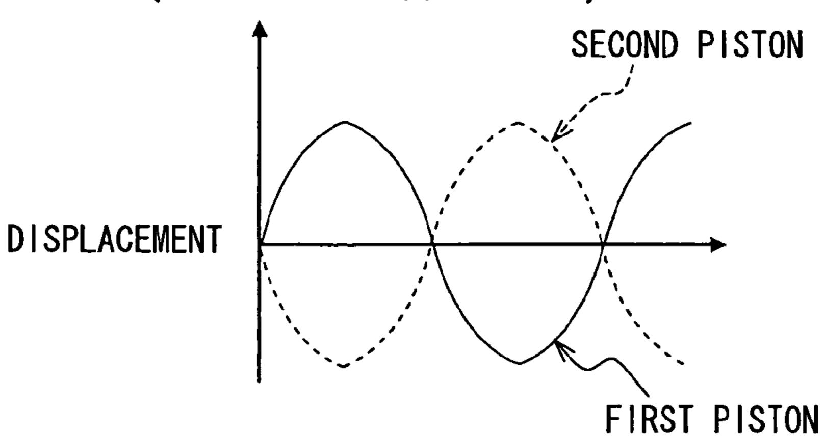
FIG. 5B PISTONS ARE OUT OF A SYNCHRONIZED CONDITION
