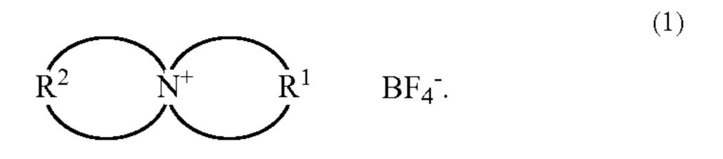
2. The electric double layer capacitor according to claim 1, wherein  $R^1$ ,  $R^2$  are both tetramethylene groups, or  $R^1$  is a tetramethylene group and  $R^2$  is a pentamethylene group.
