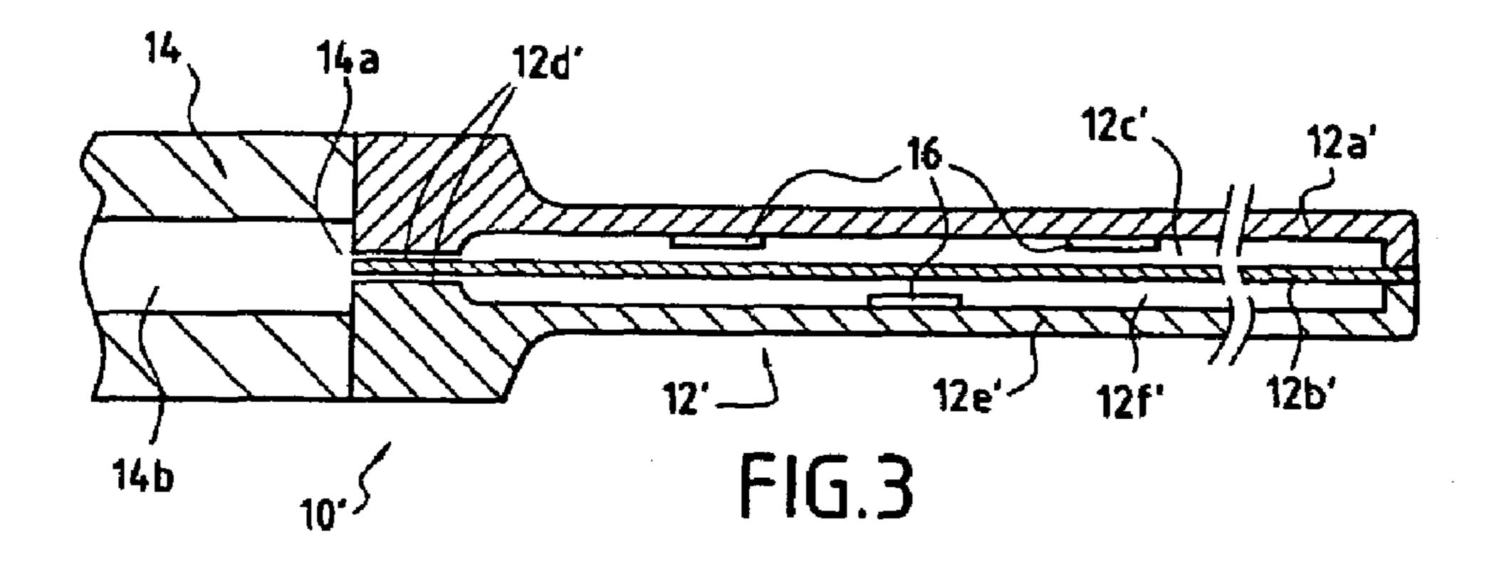
ASSEMBLY FOR THE MANUFACTURE OF A HOLLOW MECHANICAL PART BY DIFFUSION BONDING AND SUPERPLASTIC FORMING, USE OF SUCH AN ASSEMBLY AND PROCESS FOR MANUFACTURING SUCH A MECHANICAL PART
