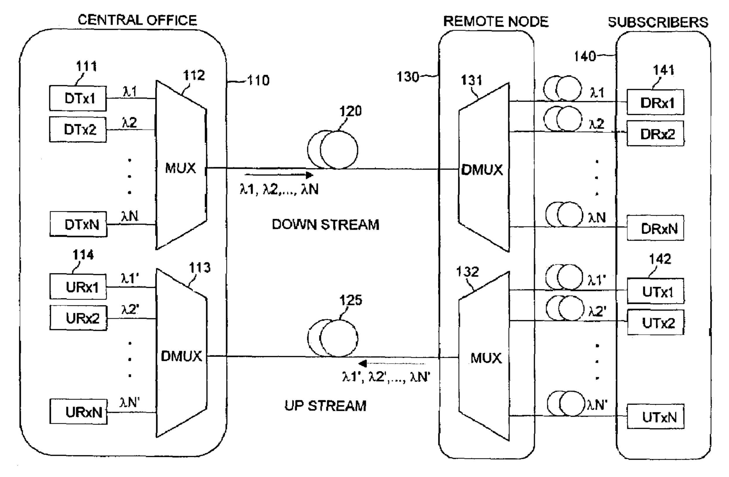
DTx:DOWNSTREAM TRANSMITTER, DRx:DOWNSTREAM RECEIVER, UTx:UPSTREAM TRANSMITTER, URx:UPSTREAM RECEIVER, MUX:MULTIPLEXER, DMUX:DEMULTIPLEXER
