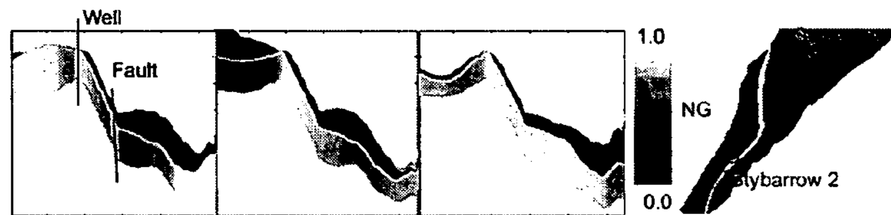
(c) elevation view of 3 realisations of 3 layers along line shown: main reservoir is third layer
