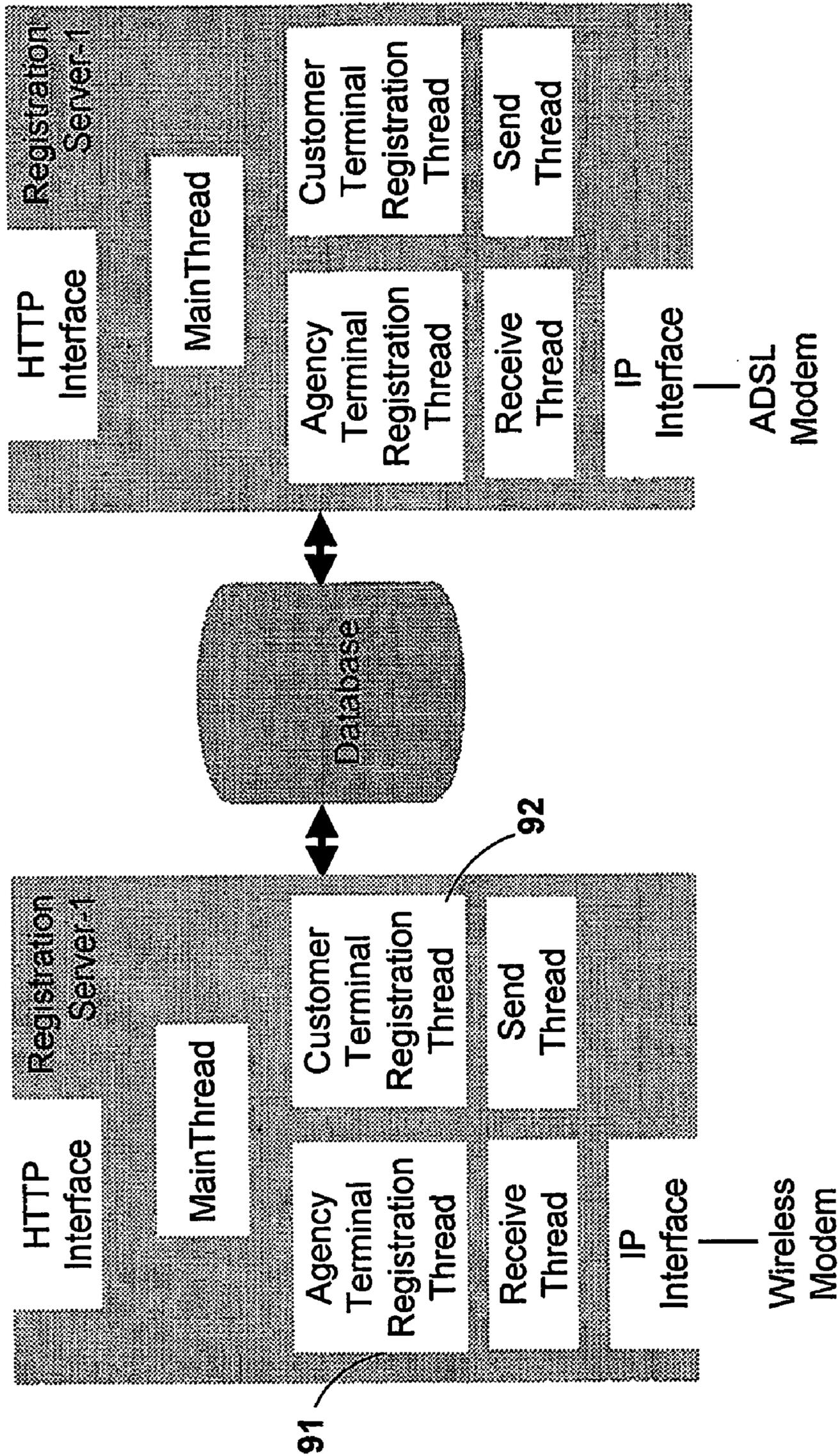
Figure 9: Registration Server Schematic
