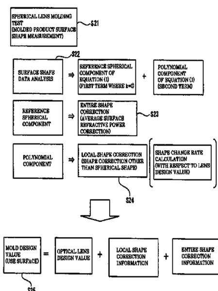
information for molding the optical lens of which curved surface is in the spherical shape. By using the correction information compiled into database, design values of the use surfaces in the upper mold and the lower mold of the mold with which the optical lens of which curved surface in the aspherical shape is molded are corrected to design them.
