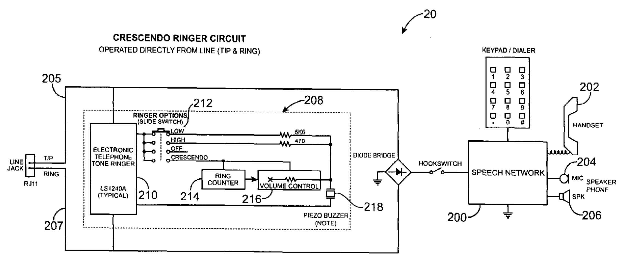
NOTE: PIEZO BUZZER CAN BE REPLACED WITH A SPEAKER
