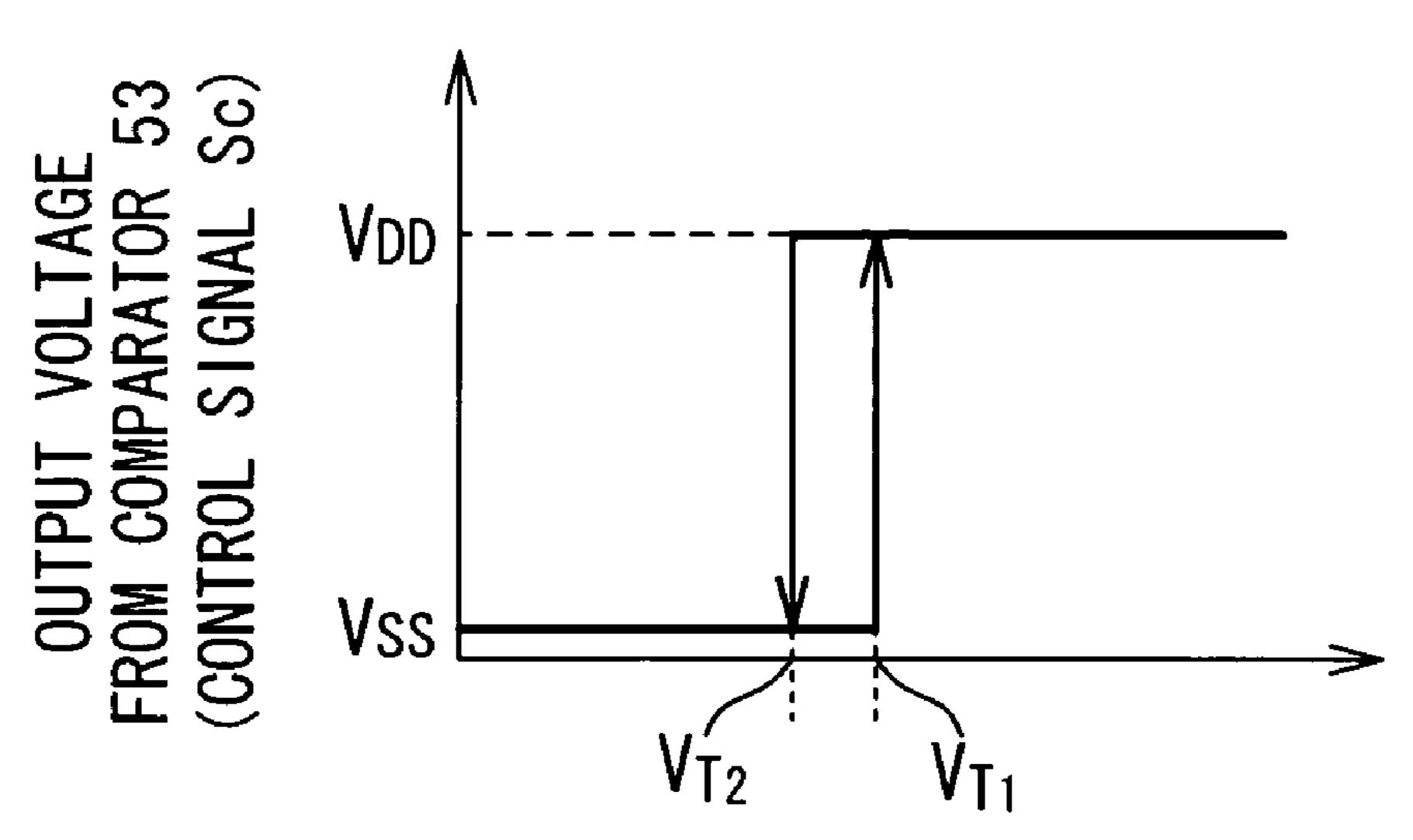
INPUT VOLTAGE TO COMPARATOR 53 (OUTPUT VOLTAGE Vo FROM COMMON MODE VOLTAGE DETECTION CIRCUIT 51) Jul. 24, 2007
