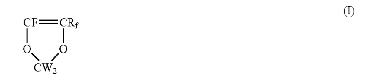
wherein  $R_f = -F$ ,  $-(O)_y C_n F_{2n+1}$  with y=0, 1 and n=1, 2, 3, 4, 5, and with W = -F,  $-C_n F_{2n+1}$ , optionally in the presence of tetrafluoroethylene and/or hexafluoropropene, and subsequent reduction of the obtained peroxidic perfluoropolyethers.
