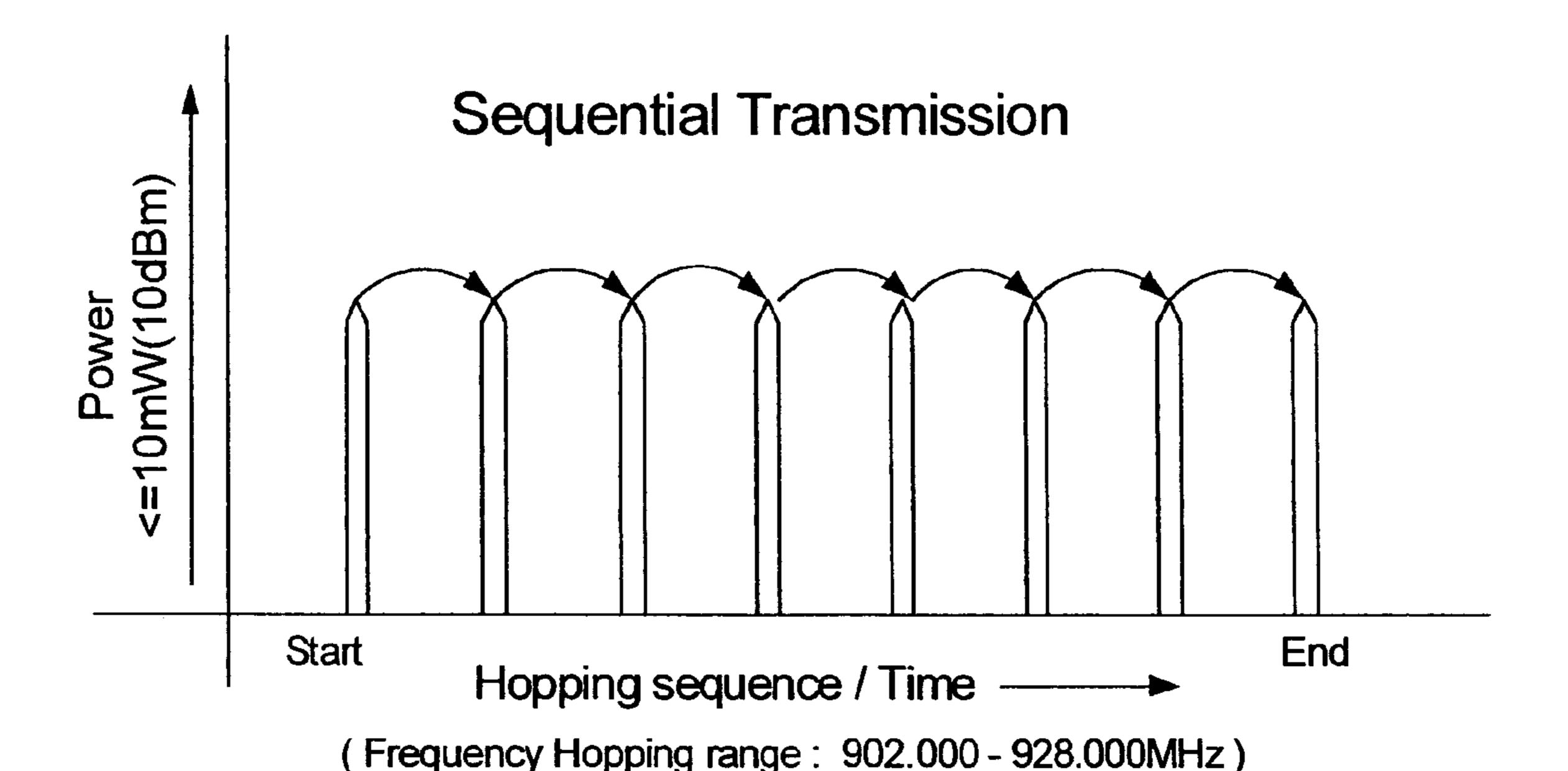
The sequential transmission for a Sequential Transmission Asynchronous Reception System ("STARS") showing eight (8) broadcasting frequencies within a selected frequency sub-band
