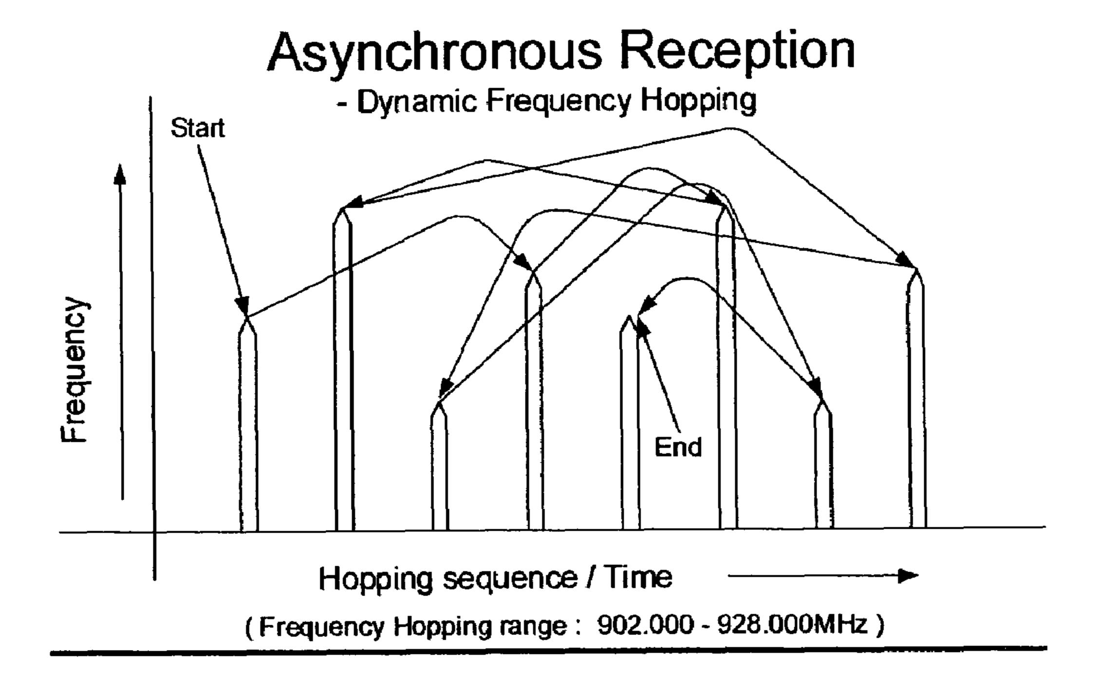
Figure 2. The mechanism for the dynamic frequency hopping in the asynchronous reception operation of the "STARS" wireless methodology
