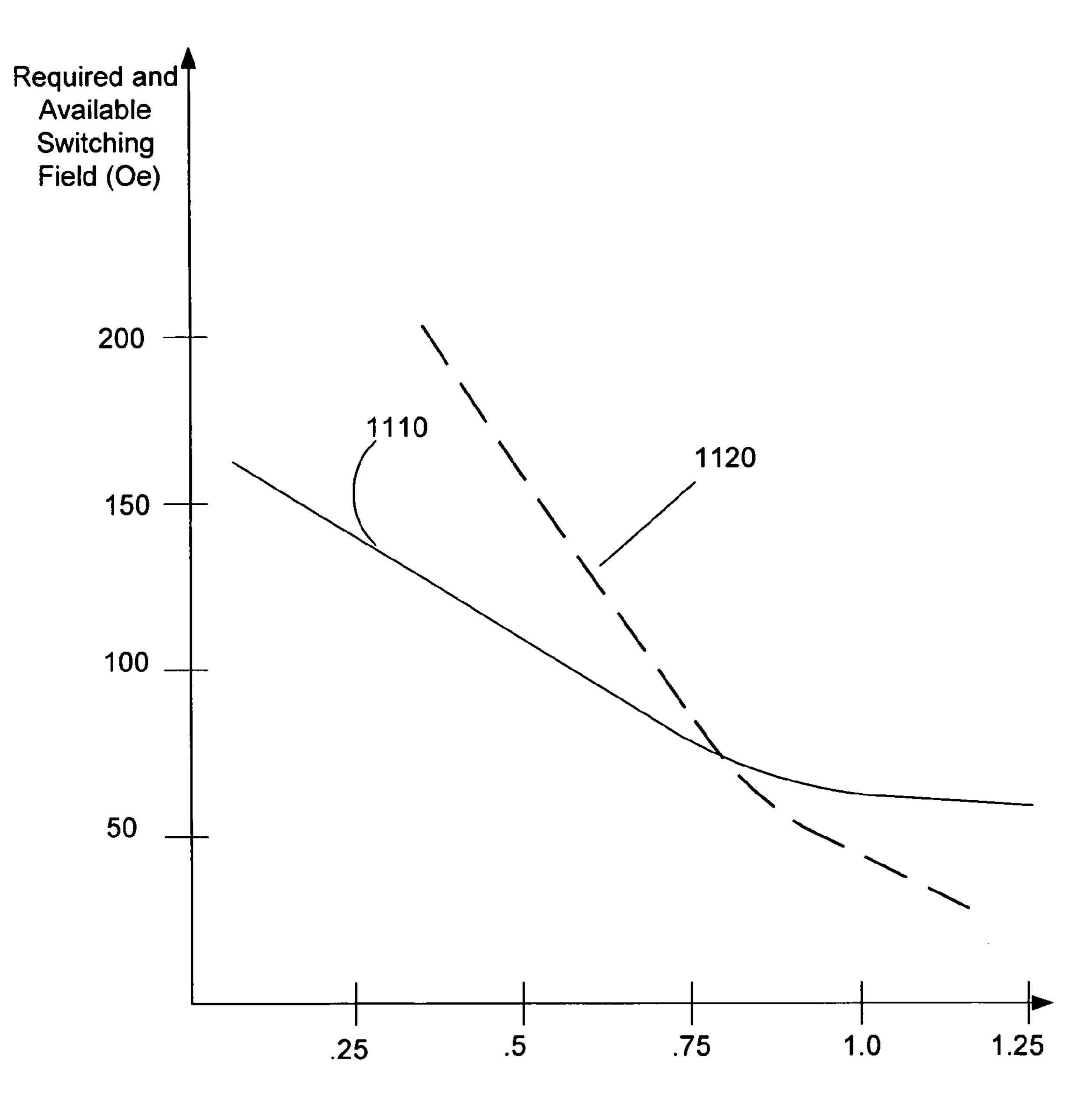
W2/W1 Ratio of Conductive Write Line and Memory Cell
