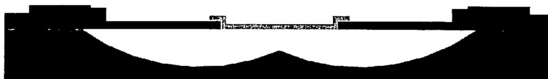
Ti/Au Evaporation (60Å/2000Å) and patterning; XeF<sub>2</sub> release
