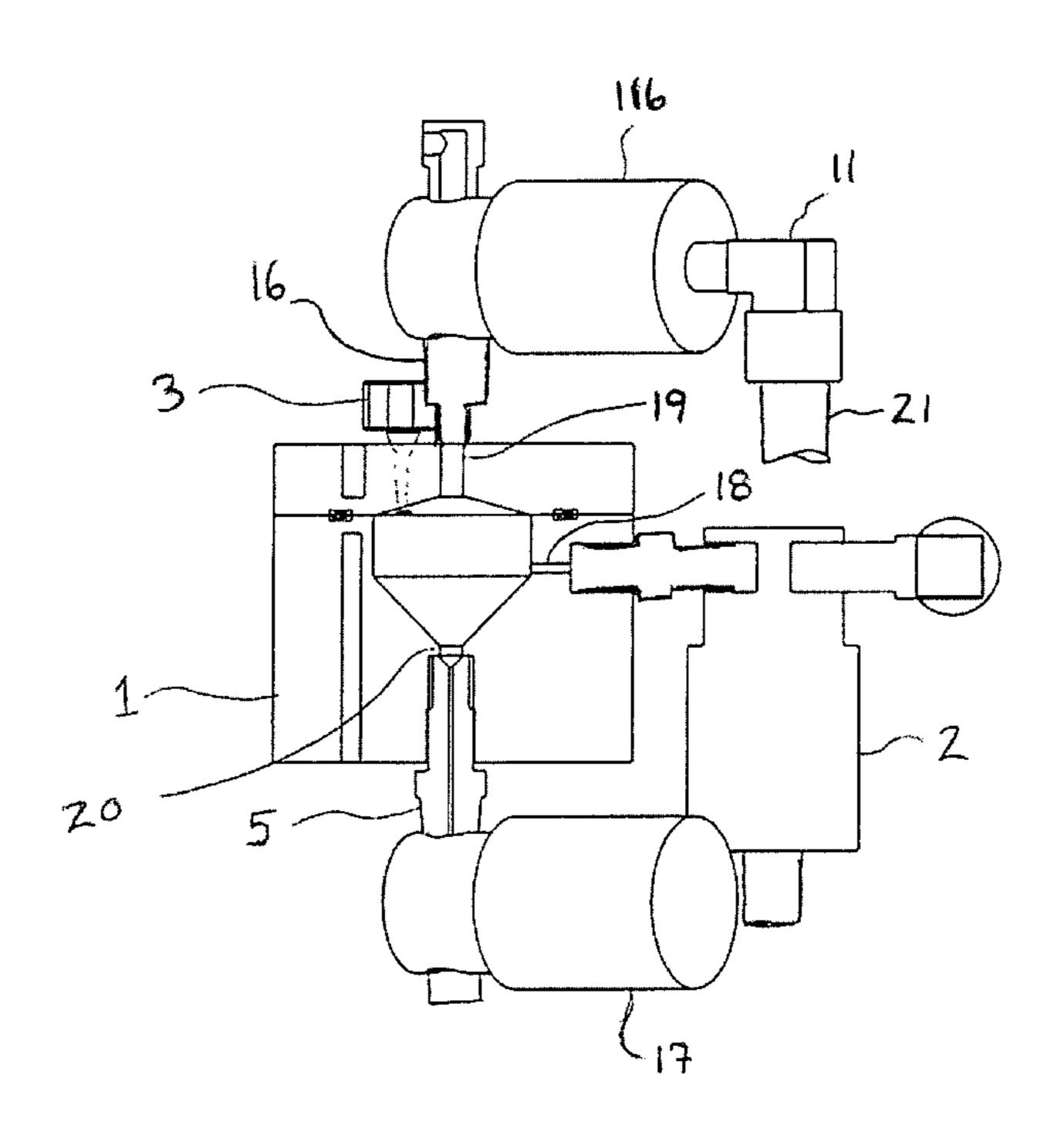
Dual Temperature, Over-Pressure Viscometer
