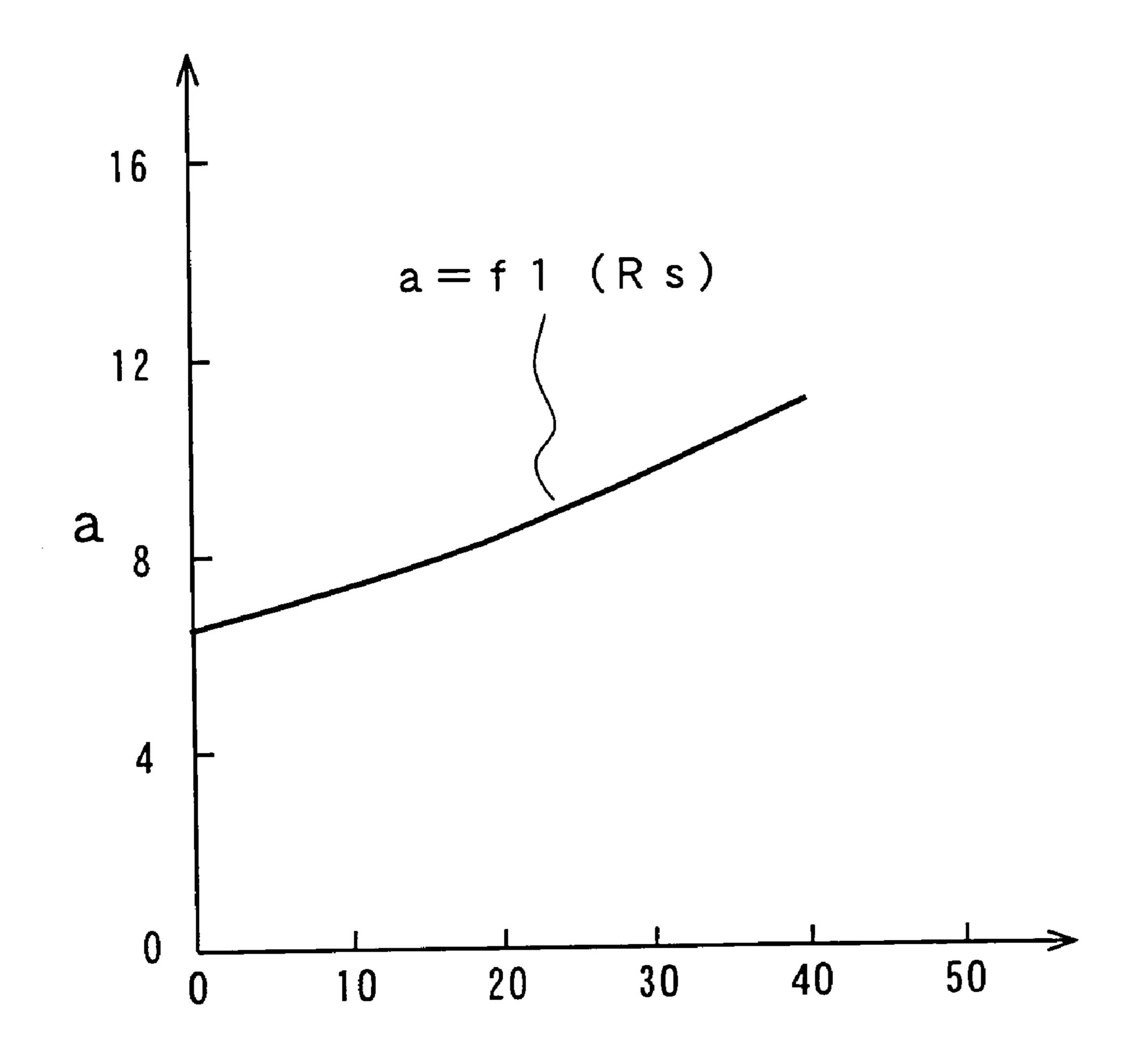
Electrode negative current rate settign value Rs(%)
