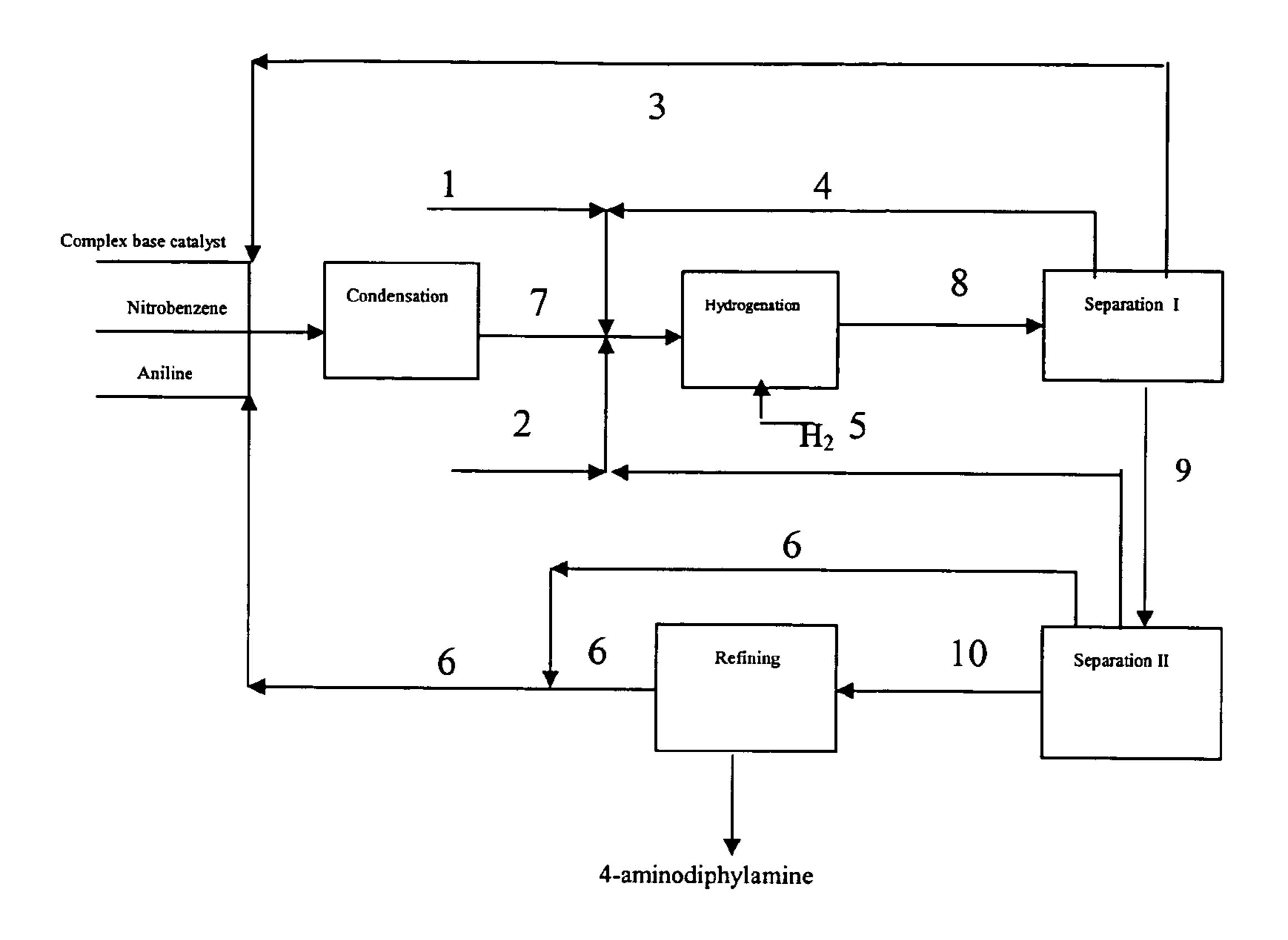
Figure 1 A flow diagram of the process for preparing 4-aminodiphylamine
