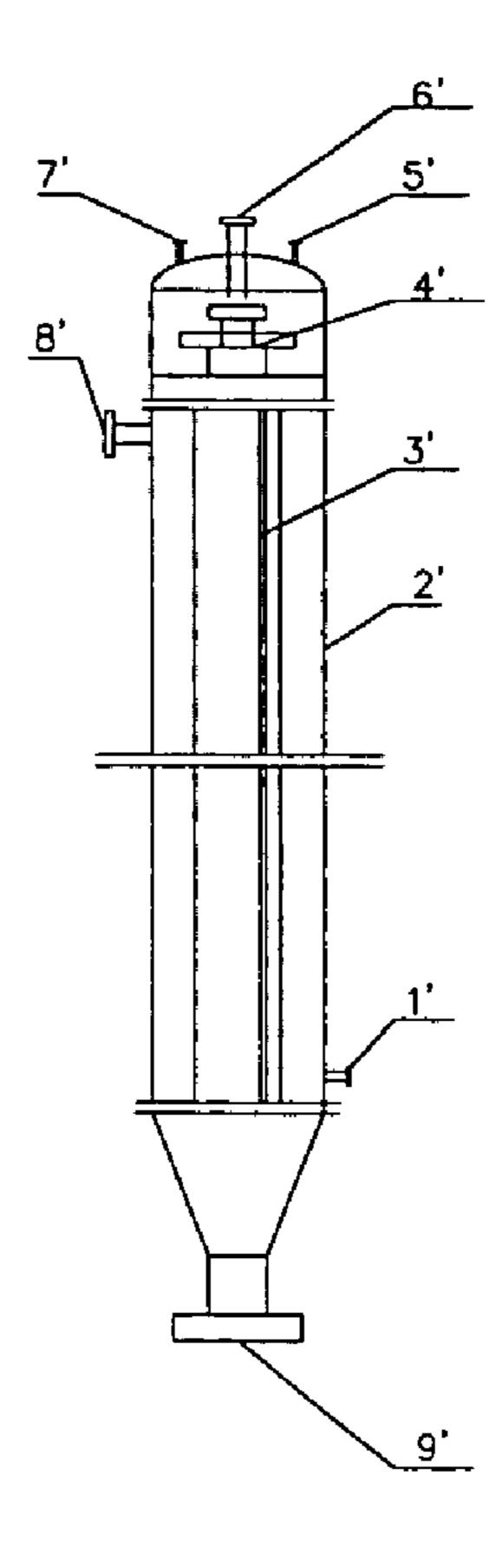
Figure 2. Schematic diagram of gas-aid falling film evaporator
