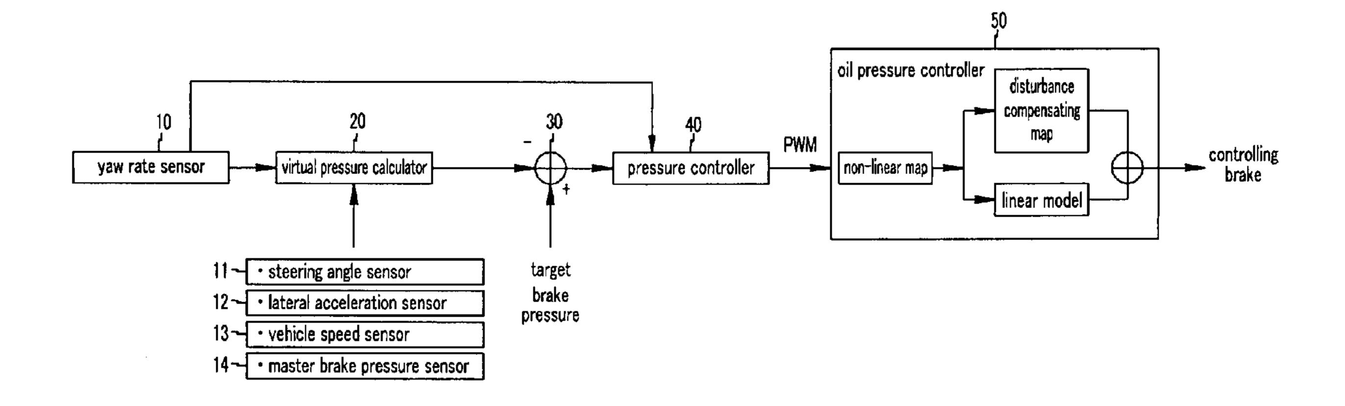
controlling brake model disturbance compensating map oil pressure controller non-linear map controller pressure brake pressure target • master brake pressure sensor lateral acceleration sensor virtual pressure calculator steering angle sensor vehicle speed sensor 24
