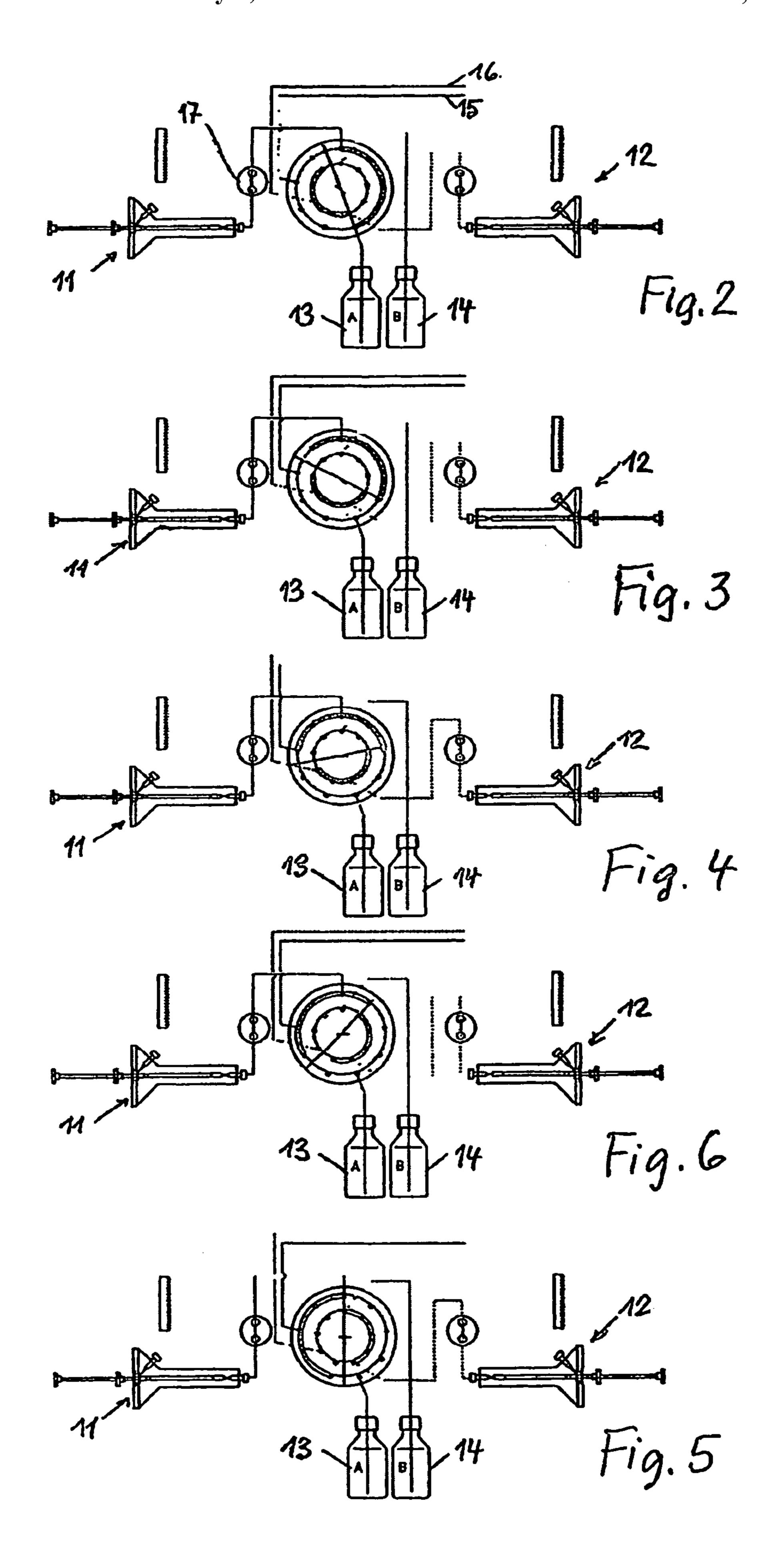
The invention is related with a rotating valve for high performance liquid chromatography (HPLC) having a stator with connections for the solvent reservoirs, pumps, chroma-
