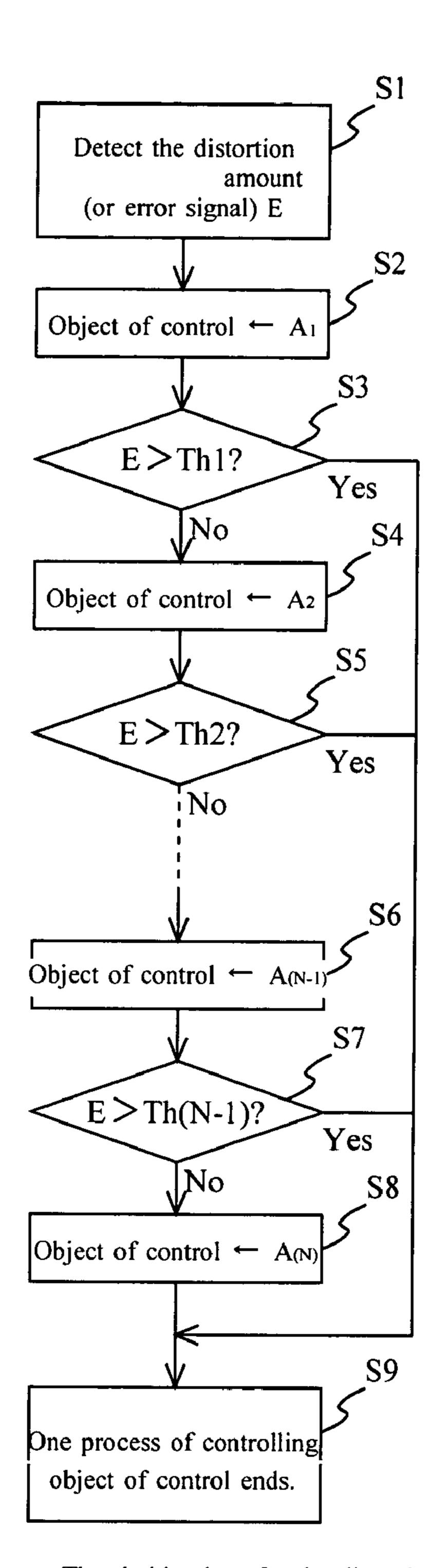
Threshold values for the distortion amount (or error signal) Th<sub>1</sub>>Th<sub>2</sub>>...>Th<sub>(N-2)</sub>>Th<sub>(N-1)</sub>
