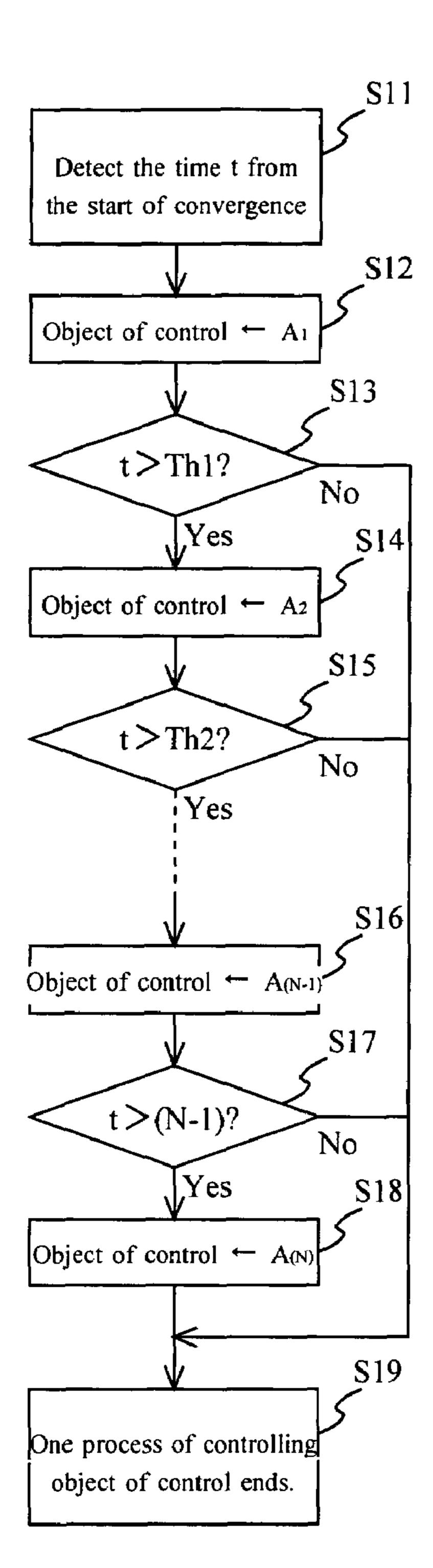
Threshold values for time from the start of convergence: T1<T2<...<T(N-2)<T(N-1)
